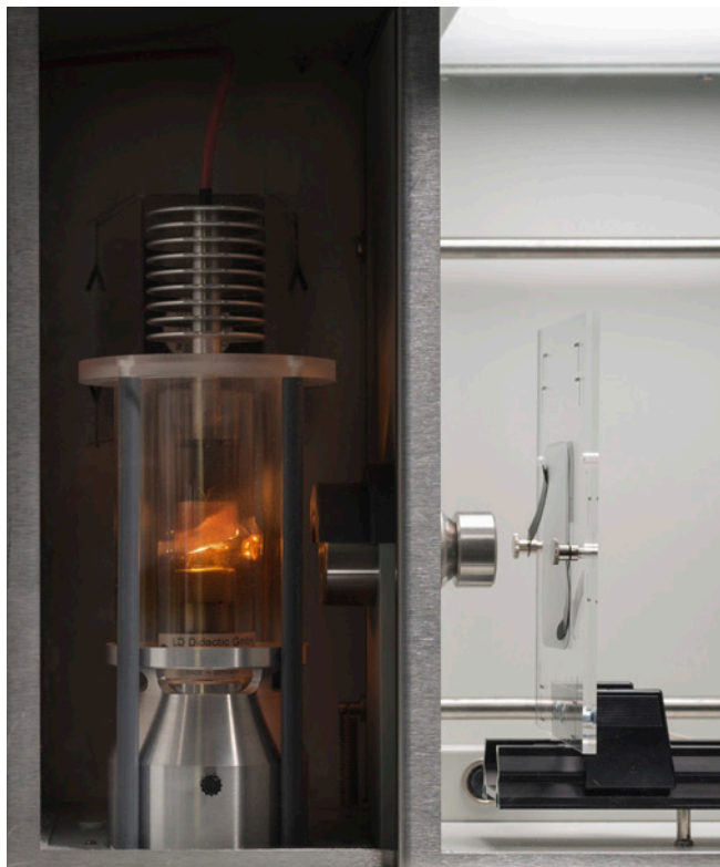
Creation of a Laue diagram on X-ray film.
