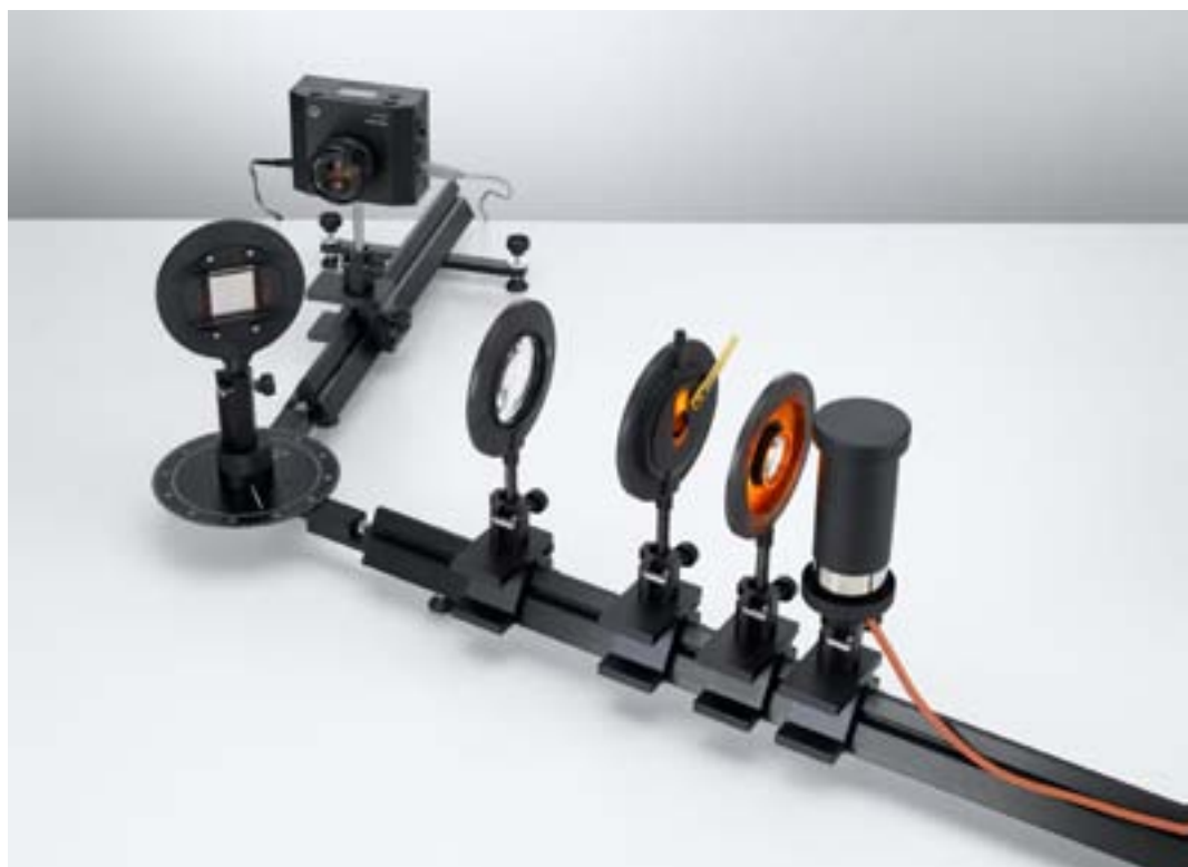
Assembling a grating spectrometer for measuring spectral lines (P5.7.2.3)
