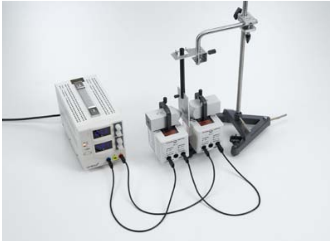
Waltenhofen's pendulum: demonstration of an eddy-current brake (P3.4.4.1)
