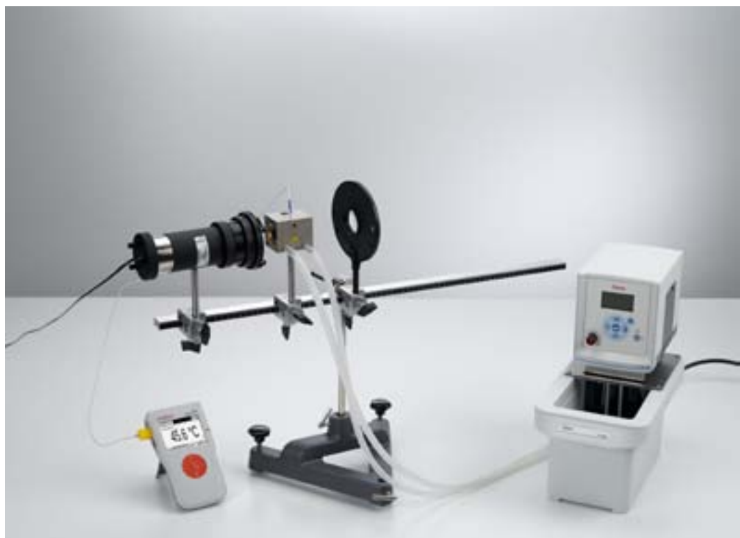
Observing the phase transition between the liquid and the gas phase at the critical point (P2.4.3.1_c)
