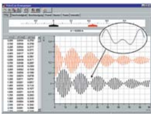
Phase shift of coupled oscillation - recorded with VideoCom (P1.5.4.2)
