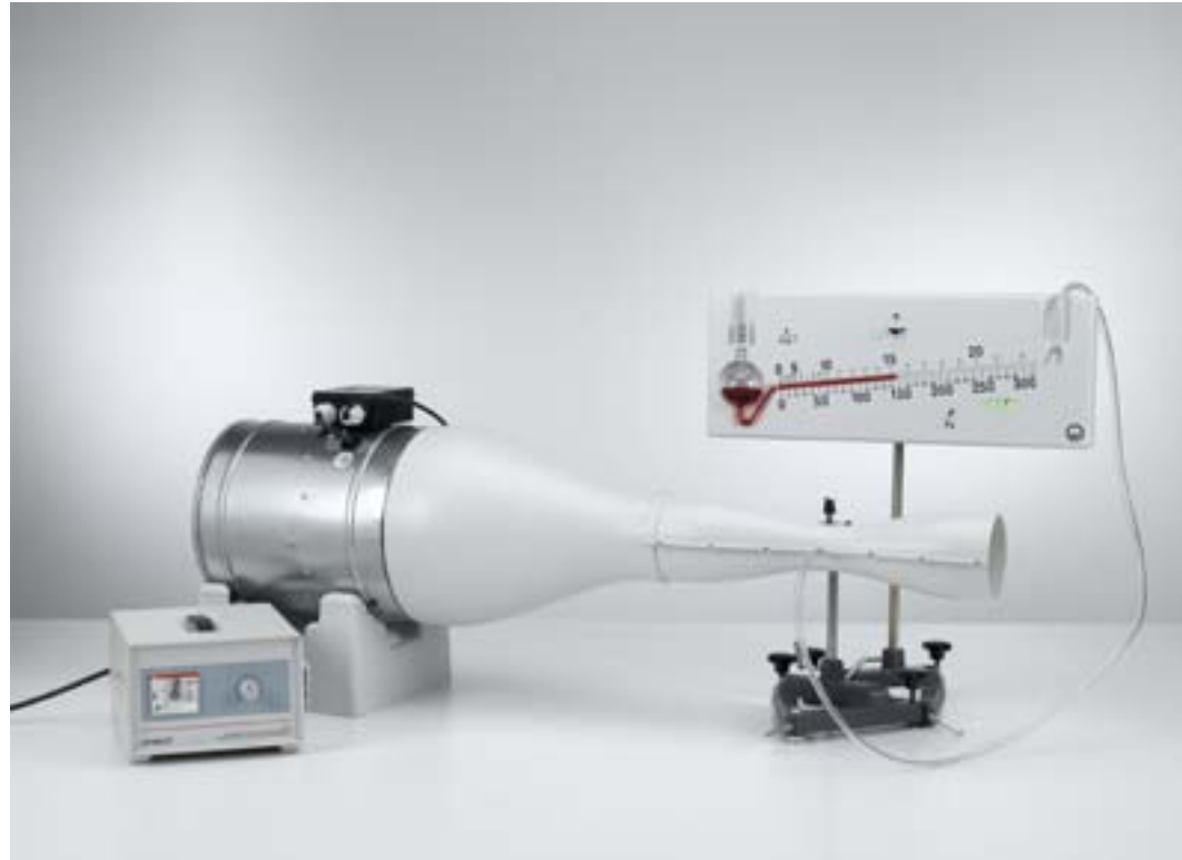
Static pressure in a reduced cross-section - Measuring the pressure with the precision manometer (P1.8.5.1)
