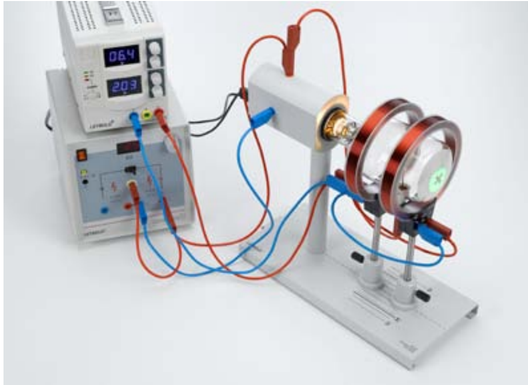
Deflection of electrons in an axial magnetic field (P3.8.3.2)
