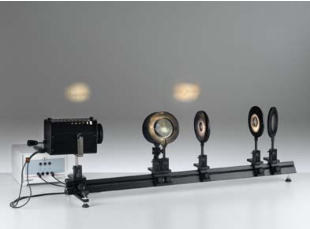
Newton's rings in transmitted and reflected white light (P5.3.3.2)
