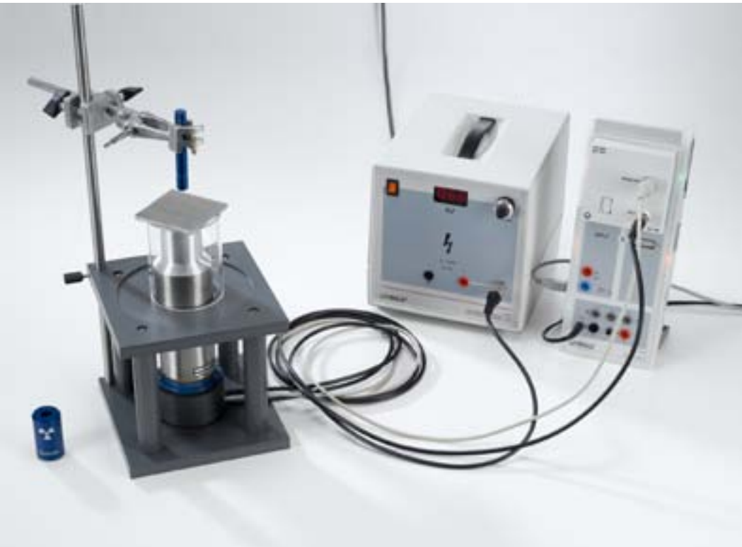
Absorption of γ radiation (P6.5.5.3)
