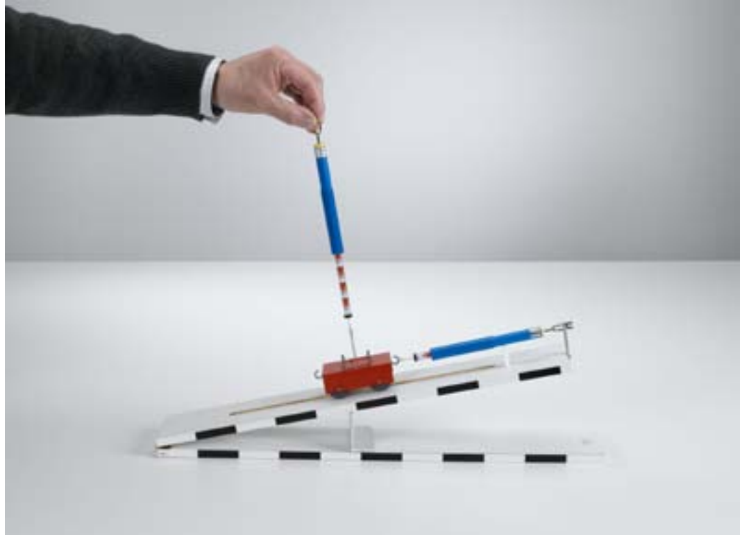
Inclined plane: force along the plane and force normal to the plane (P1.2.5.1)
