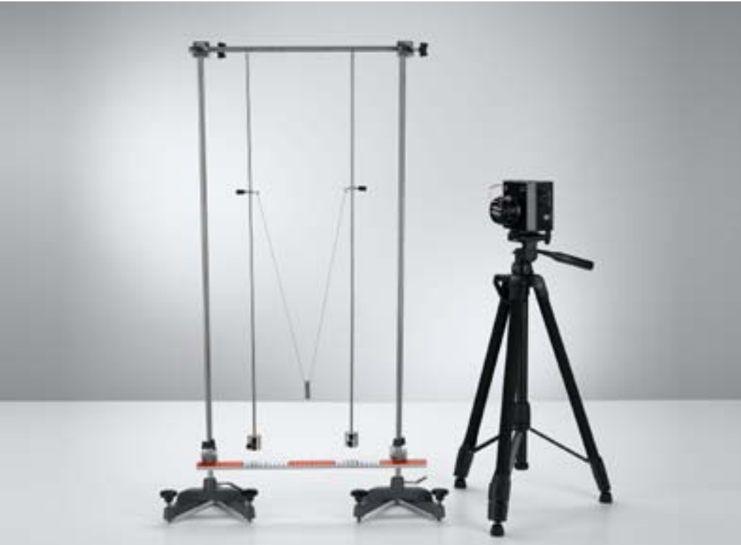
Coupled pendulum - Recording and evaluating with VideoCom (P1.5.4.2)
