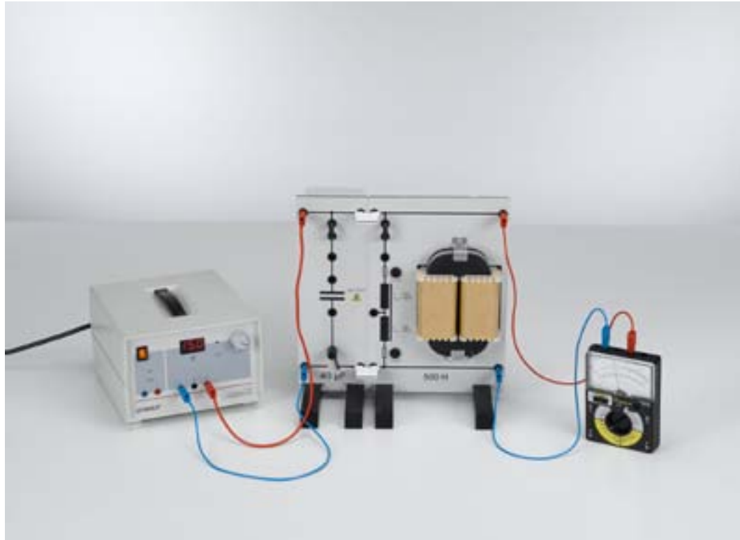
Free electromagnetic oscillations (P3.7.1.1_a)
