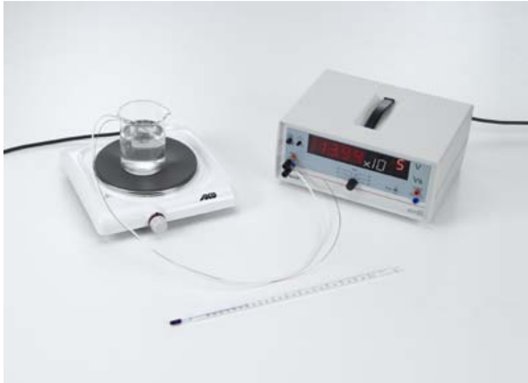
Seebeck effect: Determining the thermoelectric voltage as a function of the temperature differential (P7.2.5.1_a)
