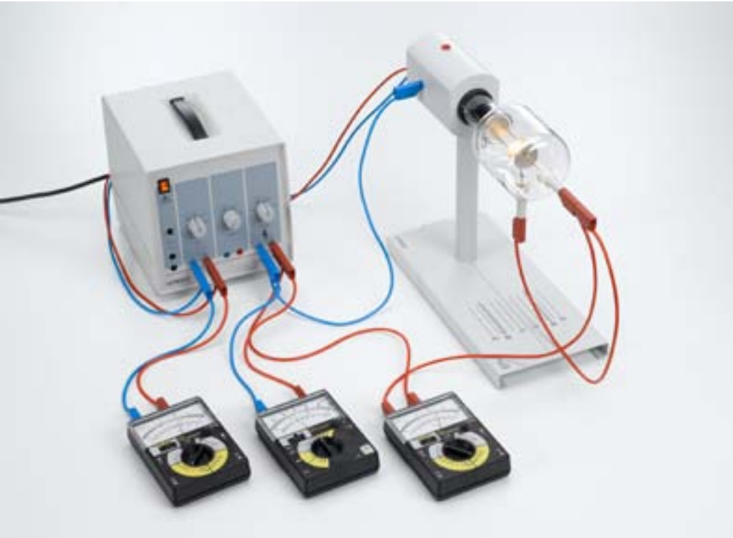
Non-spontaneous gas discharge: comparison between the charge transport in a gas triode and a high-vacuum triode (P3.9.1.1)
