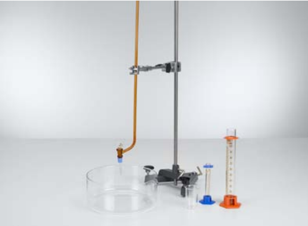
Estimating the size of oil molecules (P6.1.1.1)
