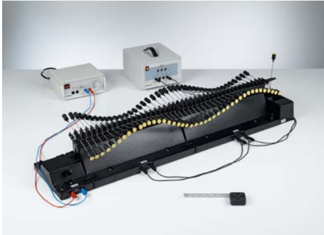
Wavelength, frequency and phase velocity of travelling waves (P1.6.2.1)
