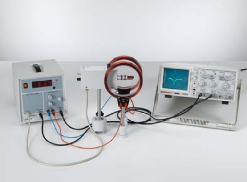
Electron spin resonance at DPPH - determining the magnetic field as a function of the resonance frequency (P6.2.6.2)
