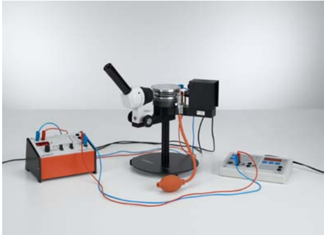
Determining the electric unit charge after Millikan and verifying the charge quantification - Measuring the suspension voltage and the falling speed (P6.1.2.1_b)
