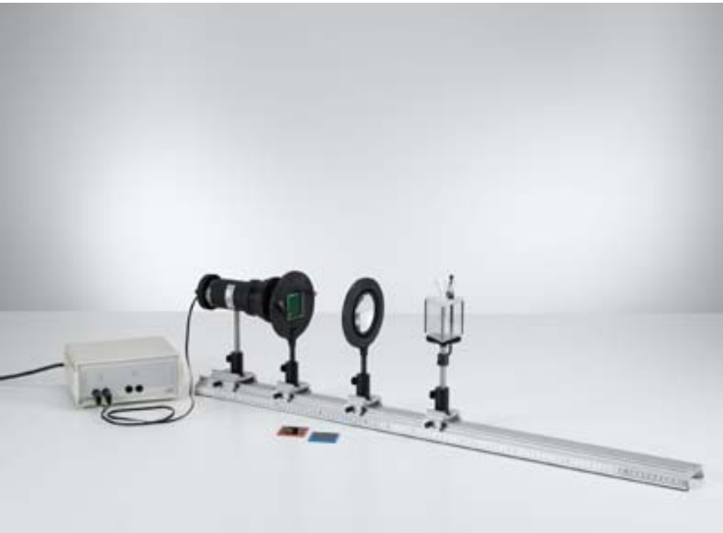
Determining the refractive index and dispersion of liquids (P5.2.1.2_b)
