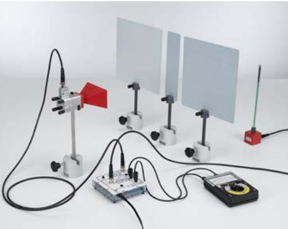
Diffraction of microwaves (P3.7.4.4)
