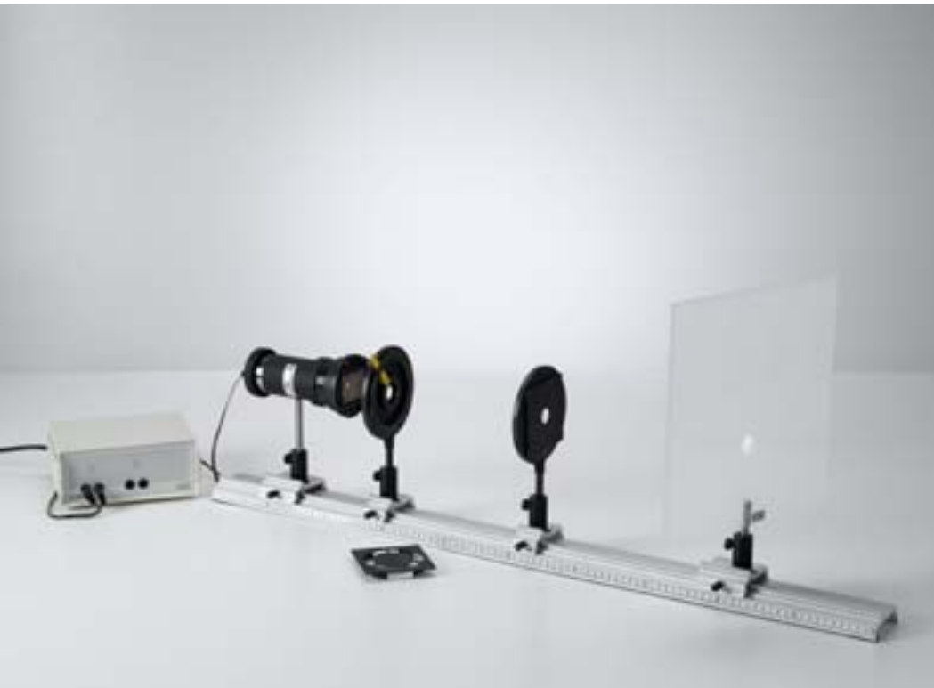
Spherical aberration in lens imaging (P5.1.3.1_b)
