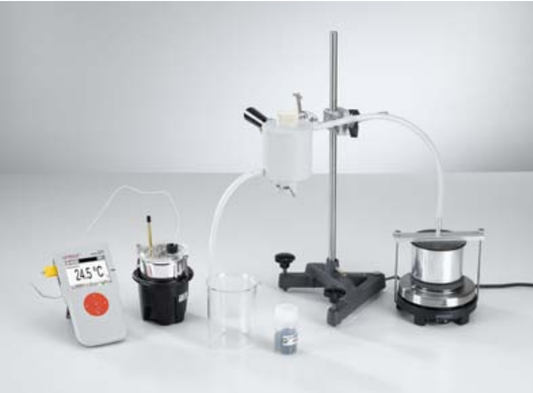
Determining the specific heat of solids (P2.3.2.1_c)
