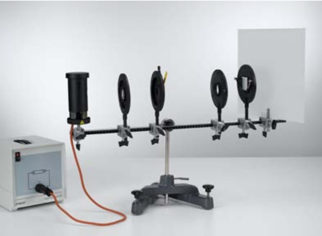
Displaying the spectral lines of inert gases and metal vapors (P6.2.2.1)
