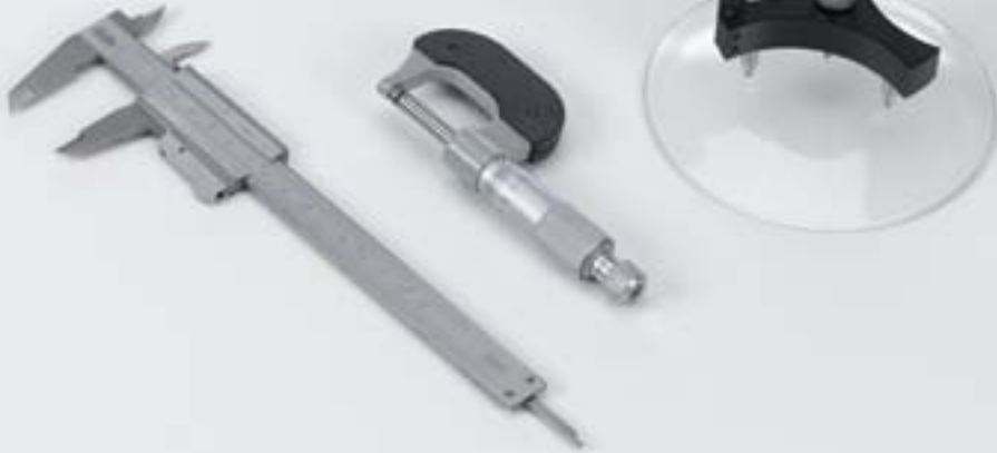
Left to right: Using a caliper gauge with vernier (P1.1.1.1), Using a micrometer screw (P1.1.1.2), Using a spherometer to determine bending radii (P1.1.1.3)
