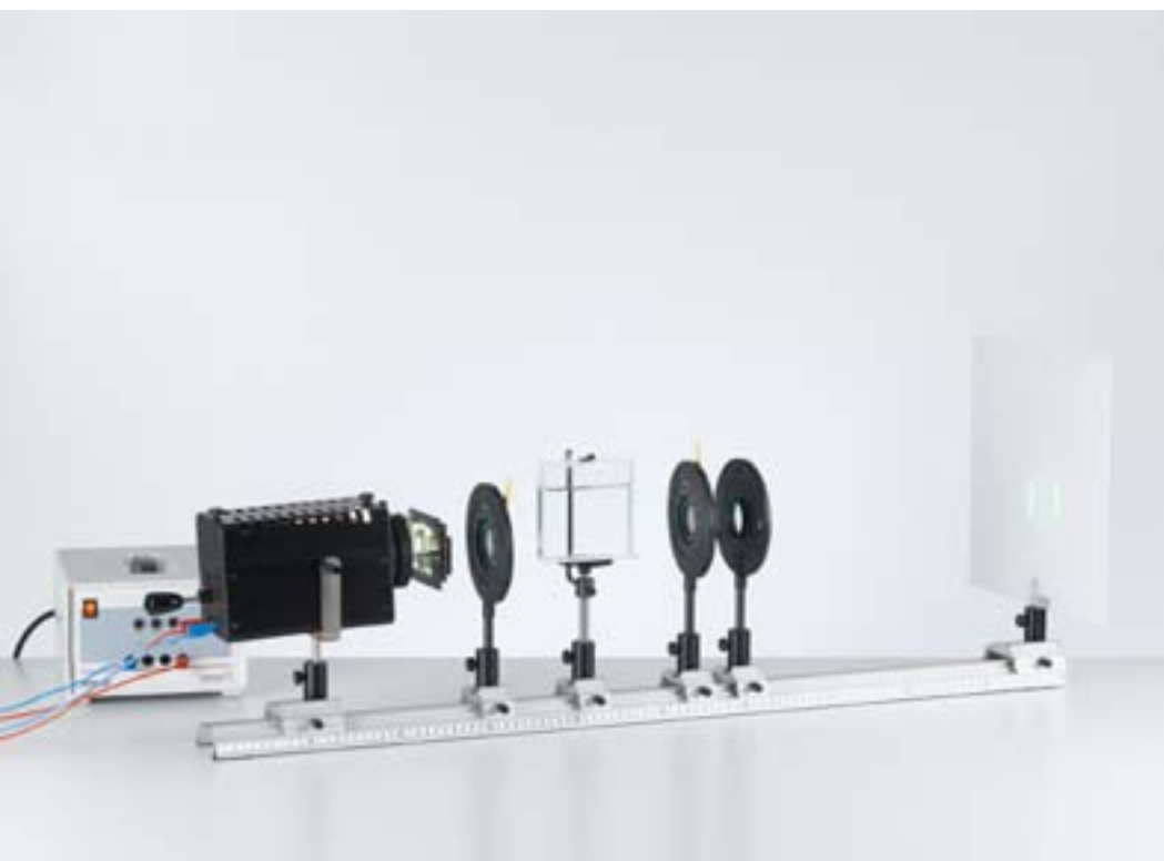
Rotation of the plane of polarization with sugar solutions (P5.4.3.2_b)
