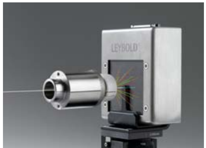
The X-ray image sensor is sensitive enough to expose the discrete reflexes behind a crystal. The zero order is shielded by a metal plate.
