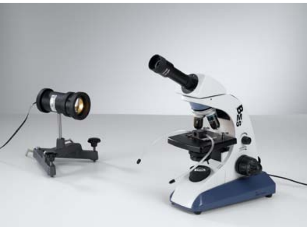
Brownian movement of smoke particles (P2.5.1.1)
