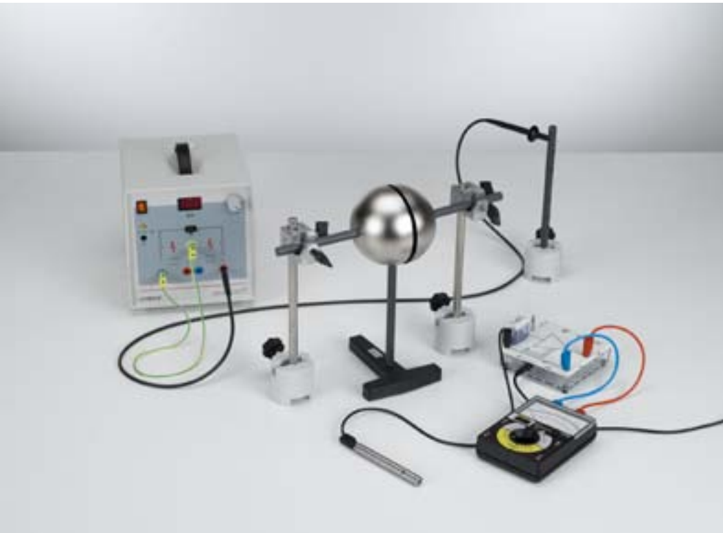
Electrostatic induction with the hemispheres after Cavendish (P3.1.5.2)
