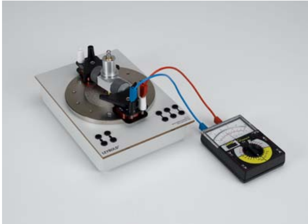
Simple induction experiments with electromagnetic rotors and stators (P3.5.1.2)
