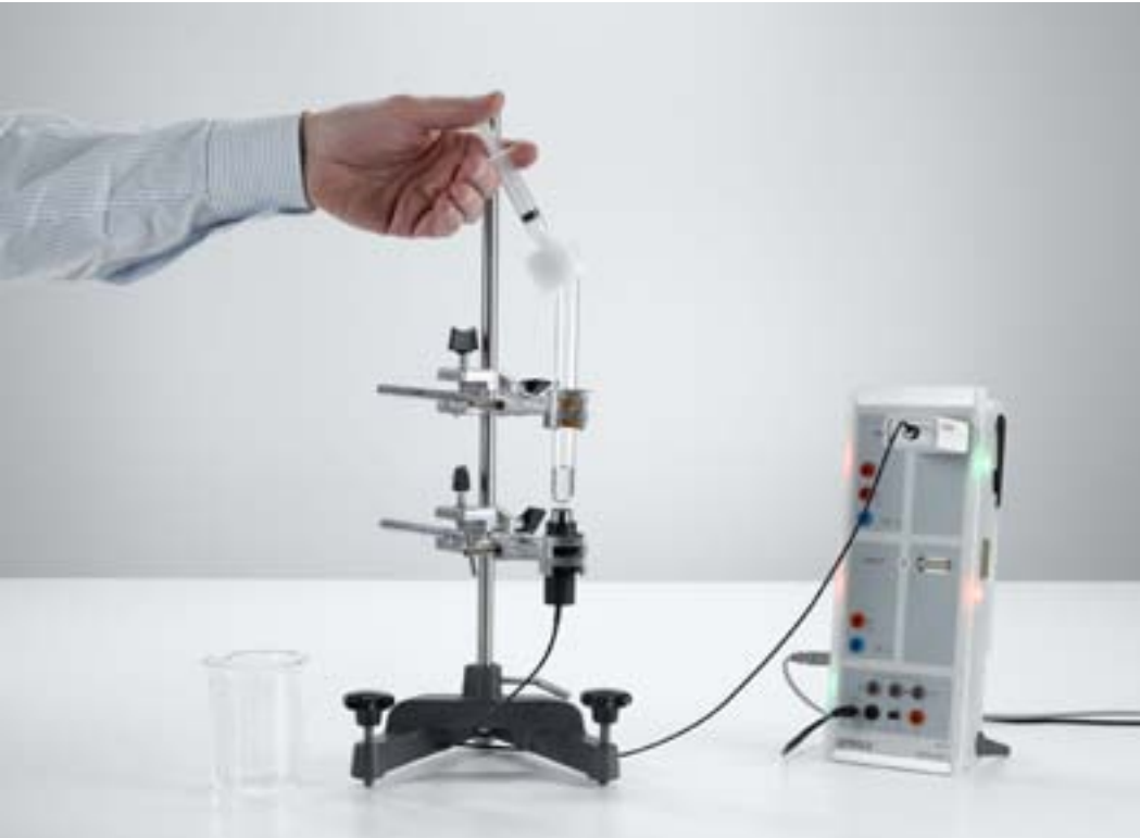
Determining the half-life of Cs-137 - Recording and evaluating the decay curve with CASSY (P6.4.3.4)
