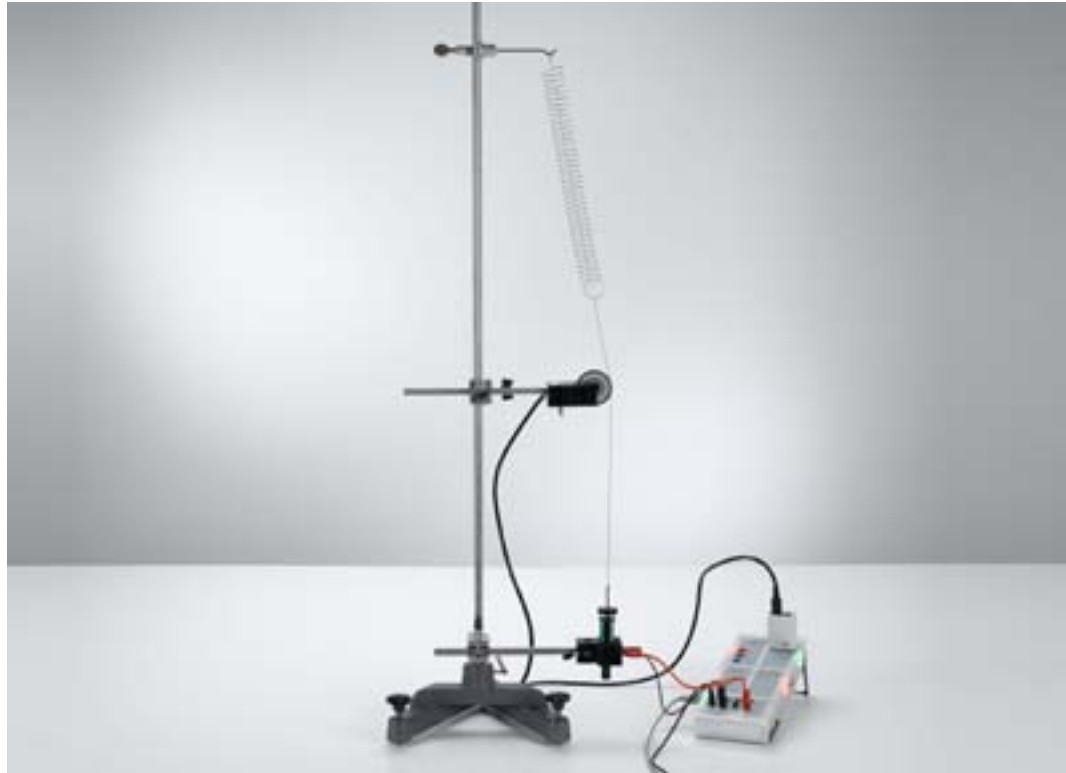
Oscillations of a spring pendulum – Recording the path, velocity and acceleration with CASSY (P1.5.2.1)
