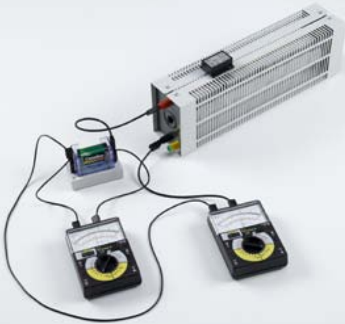
Determining the internal resistance of a battery (P4.1.1.1)
