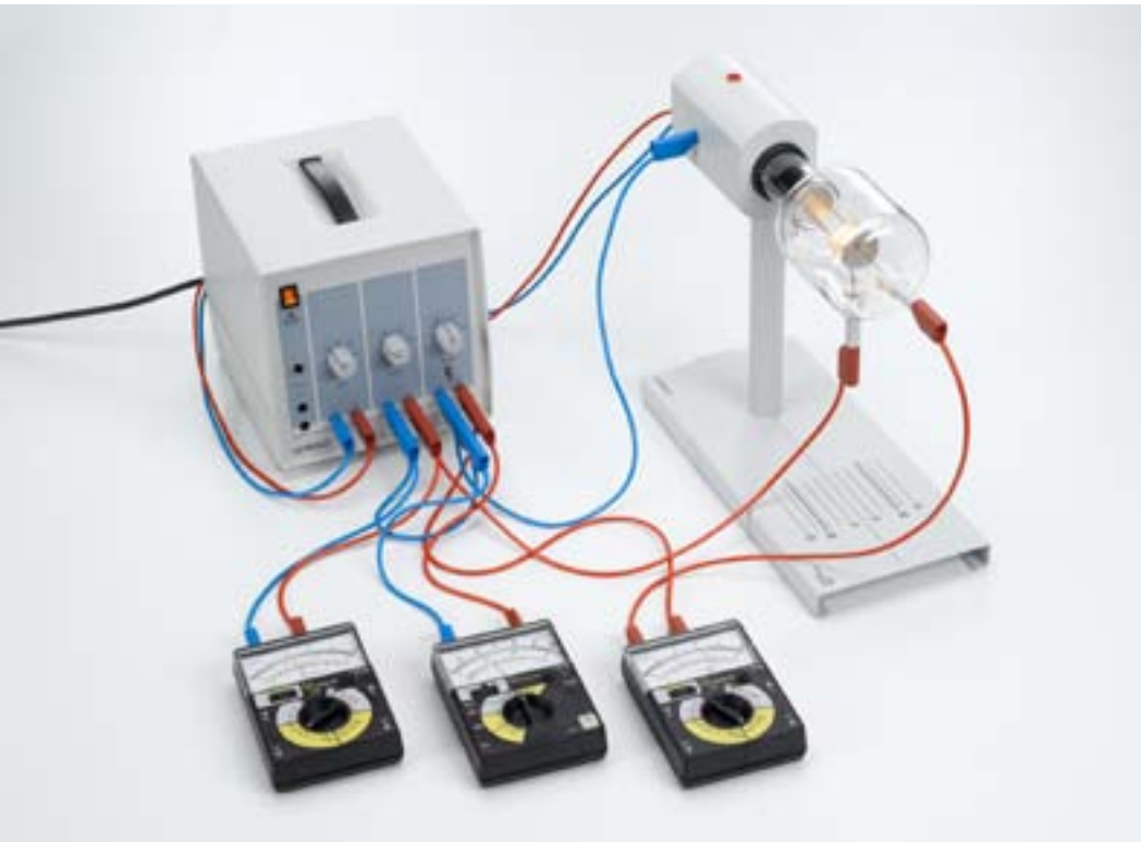
Recording the characteristic field of a tube triode (P3.8.2.1)
