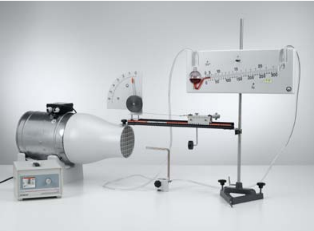
Measuring the air resistance as a function of the wind speed - Measuring the wind speed with the precision manometer (P1.8.6.1)
