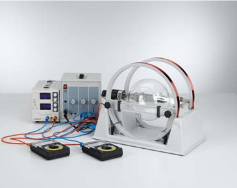
Determining the specific charge of the electron (P6.1.3.1)
