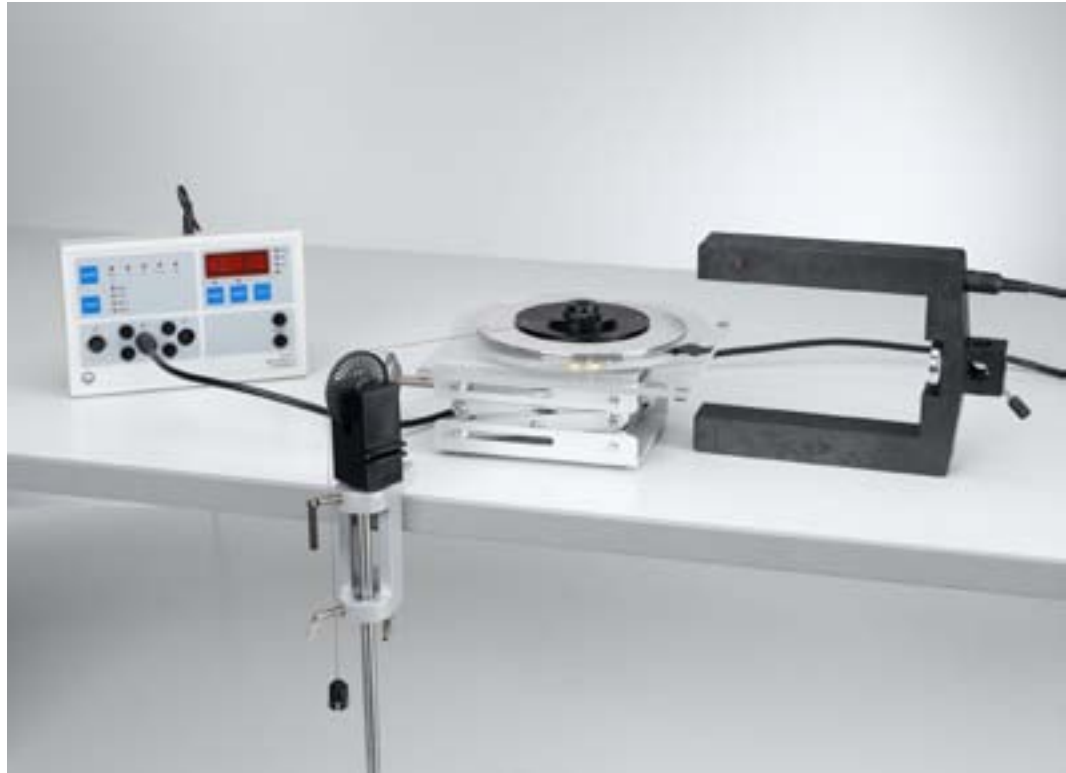
Path-time diagrams of rotational motions - Time measurement with the counter (P1.4.1.1_a)
