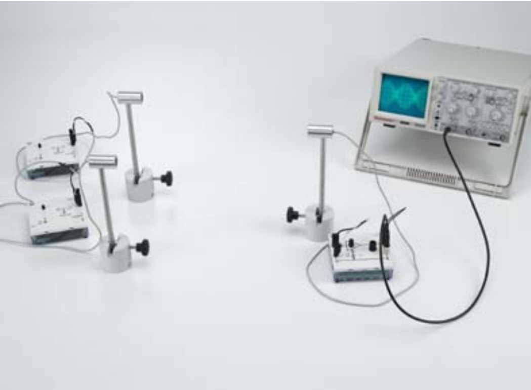
Beating of ultrasonic waves (P1.7.5.1)
