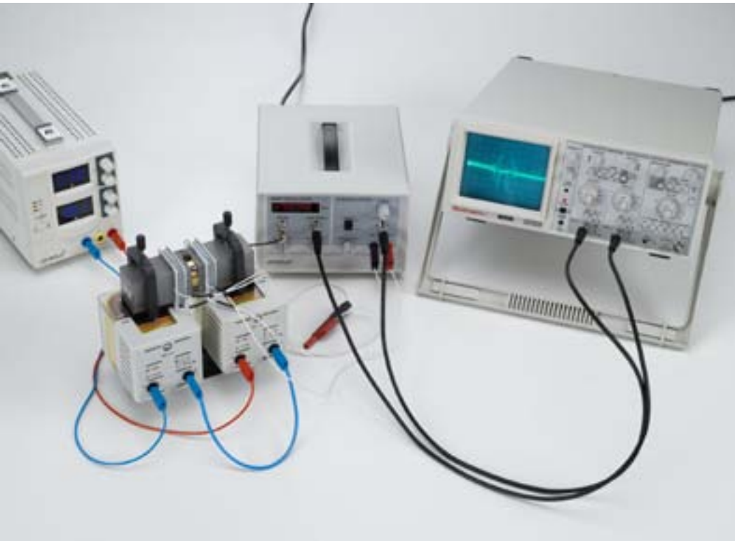
Nuclear magnetic resonance in polystyrene, glycerin and Teflon (P6.5.3.1_a)
