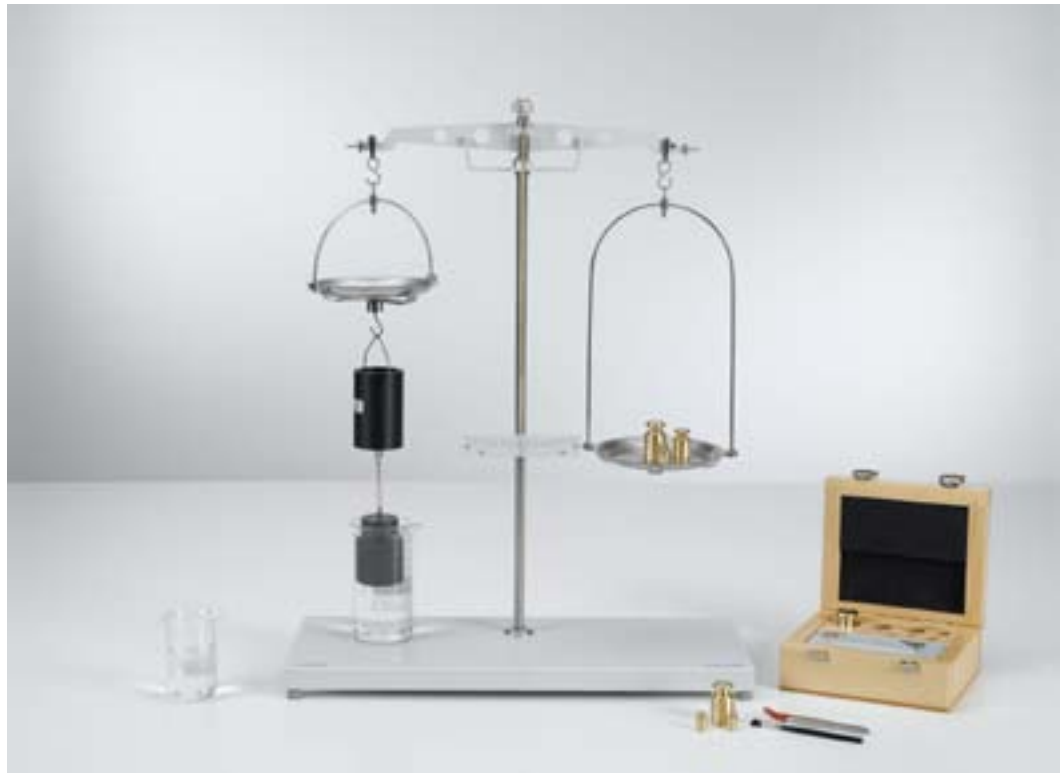
Confirming Archimedes' principle (P1.8.2.1)
