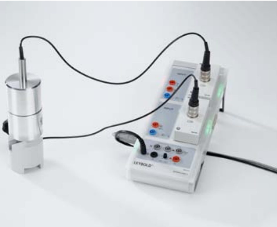
Detection of Muons (P6.6.2.1)
