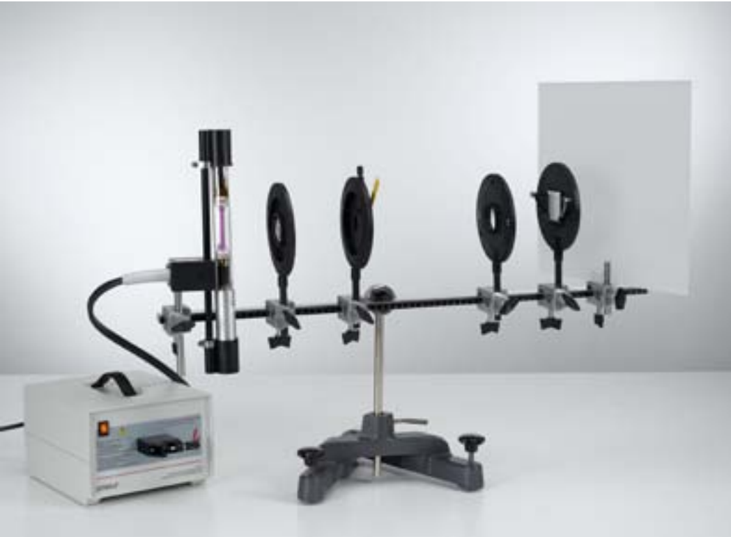
Determining the wavelengths H_{\alpha} , H_{\beta} and H_{\gamma} from the Balmer series of hydrogen (P6.2.1.1)
