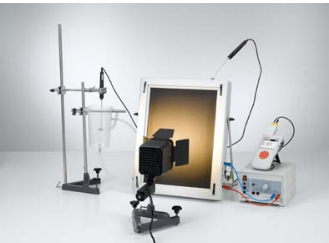
Determining the efficiency of a solar collector as a function of the throughput volume of water (P2.2.2.1_b)
