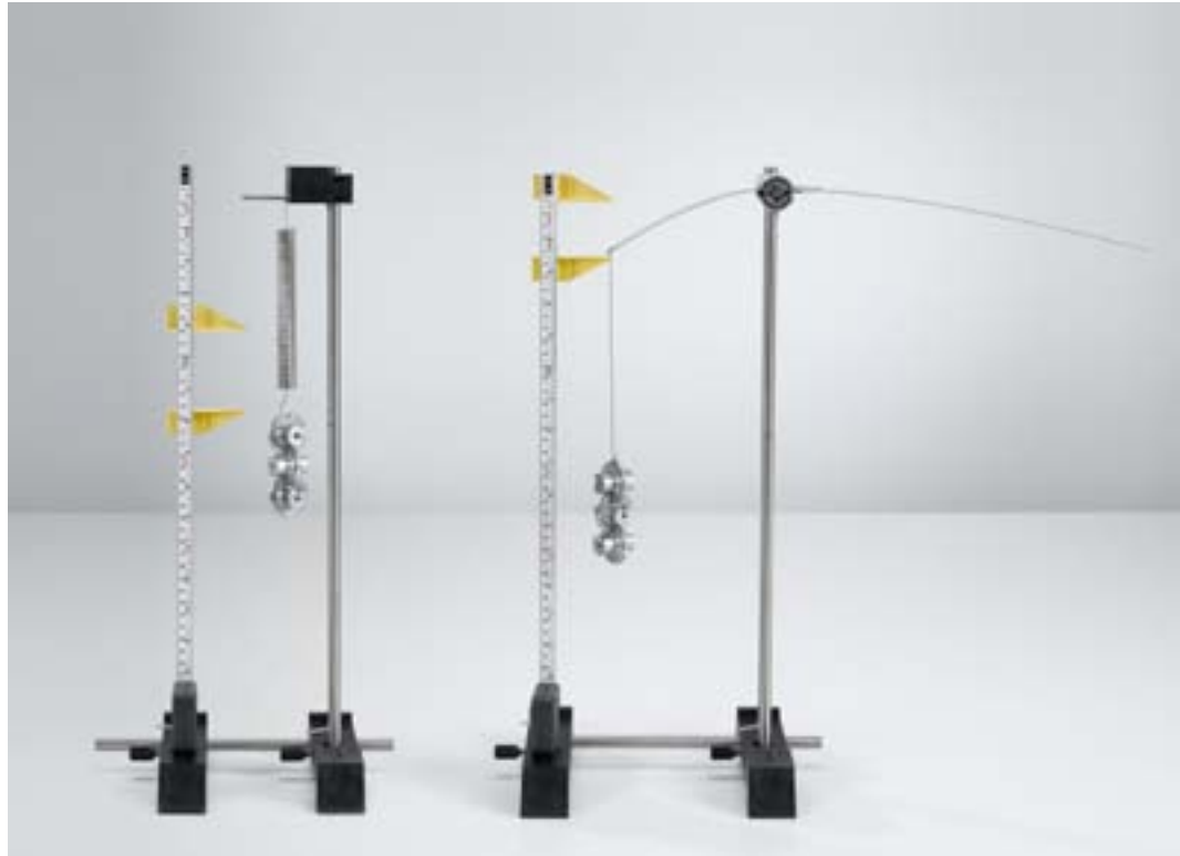
Left: Expansion of a helical spring (P1.2.1.1), Right: Bending of a leaf spring (P1.2.1.2)
