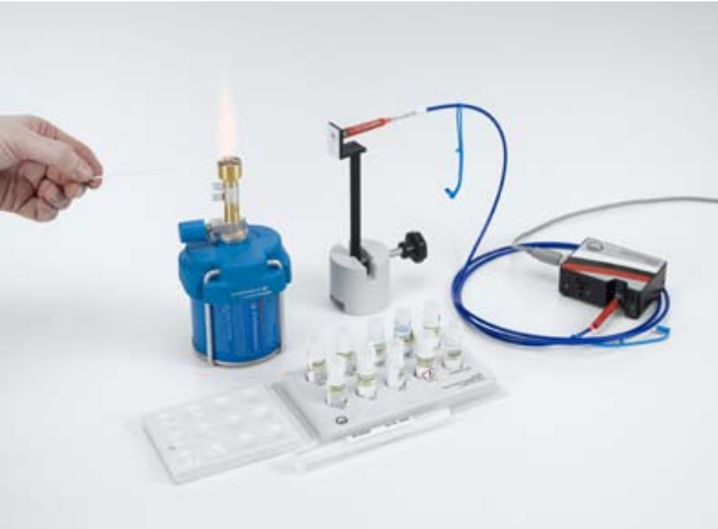
Recording the emission spectra of flame colouration (P6.2.2.4)
