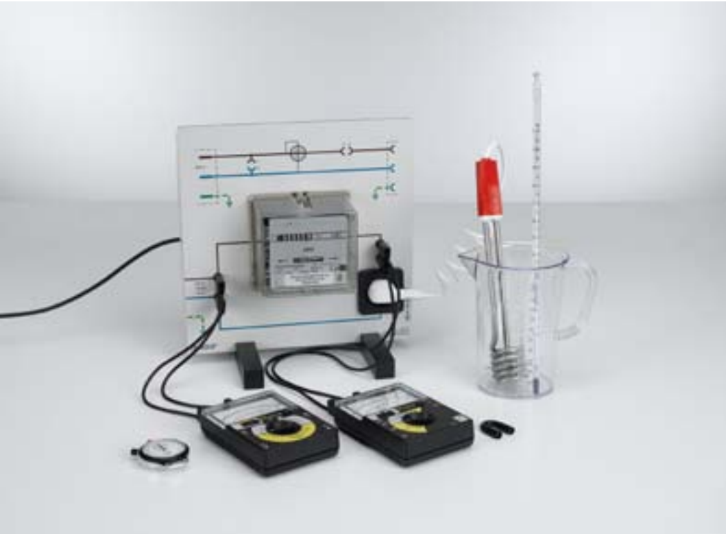
Determining the electric work of an immersion heater using an AC power meter (P3.6.6.2)
