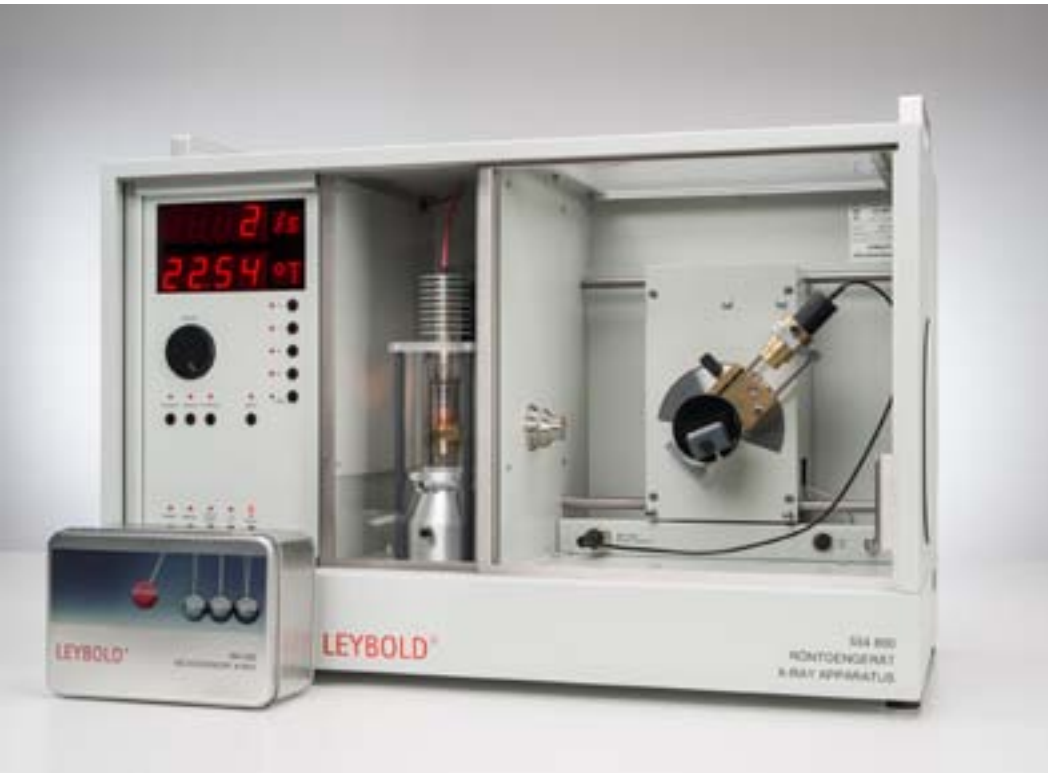
High-resolution fine structure of the characteristic X-ray radiation of a molybdenum anode (P6.3.6.11)
