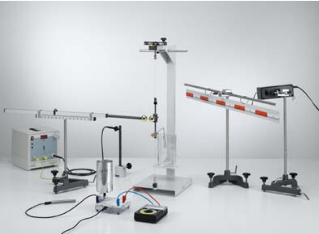
Confirming Coulomb's law - Measuring with the torsion balance, Schürholz design (P3.1.2.1)
