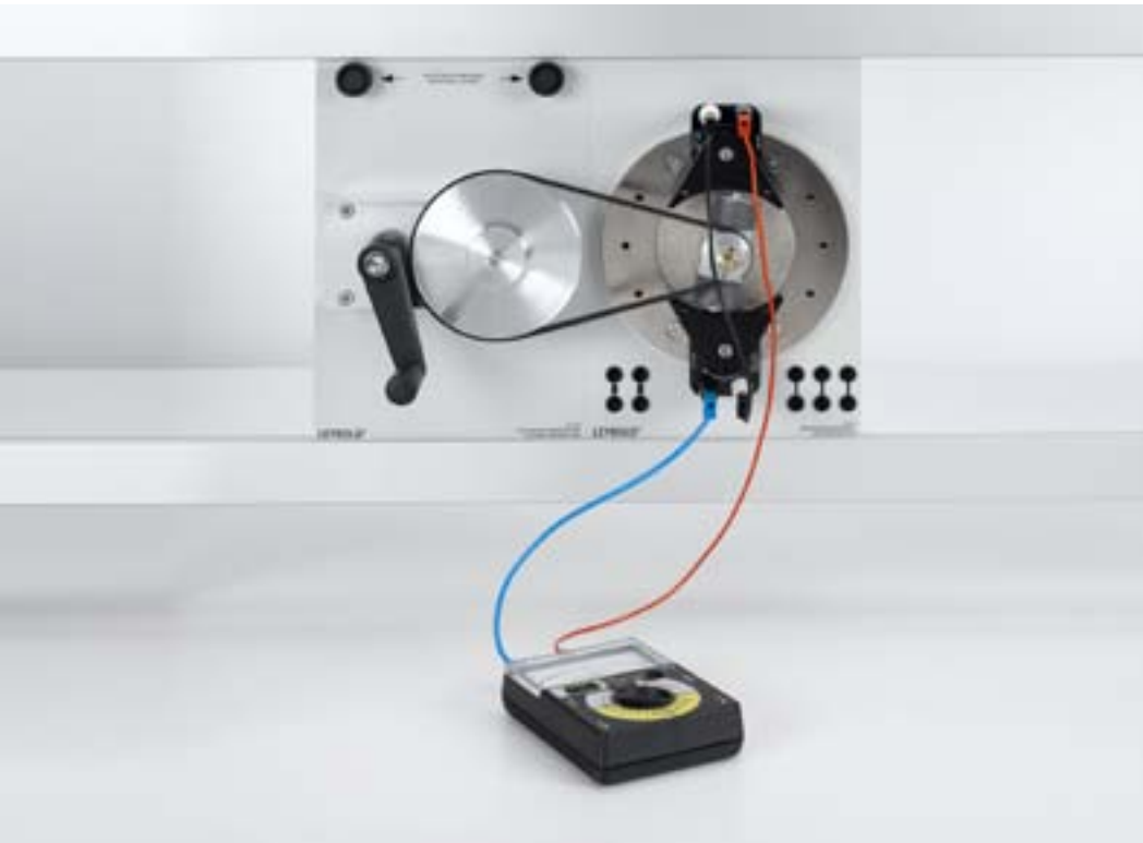
Generating AC voltage using a revolving-field generator and a stationary-field generator (P3.5.2.1_b)
