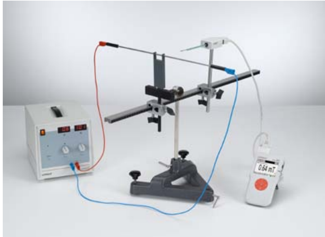
Measuring the magnetic field for a straight conductor and on circular conductor loops (P3.3.4.1_b)
