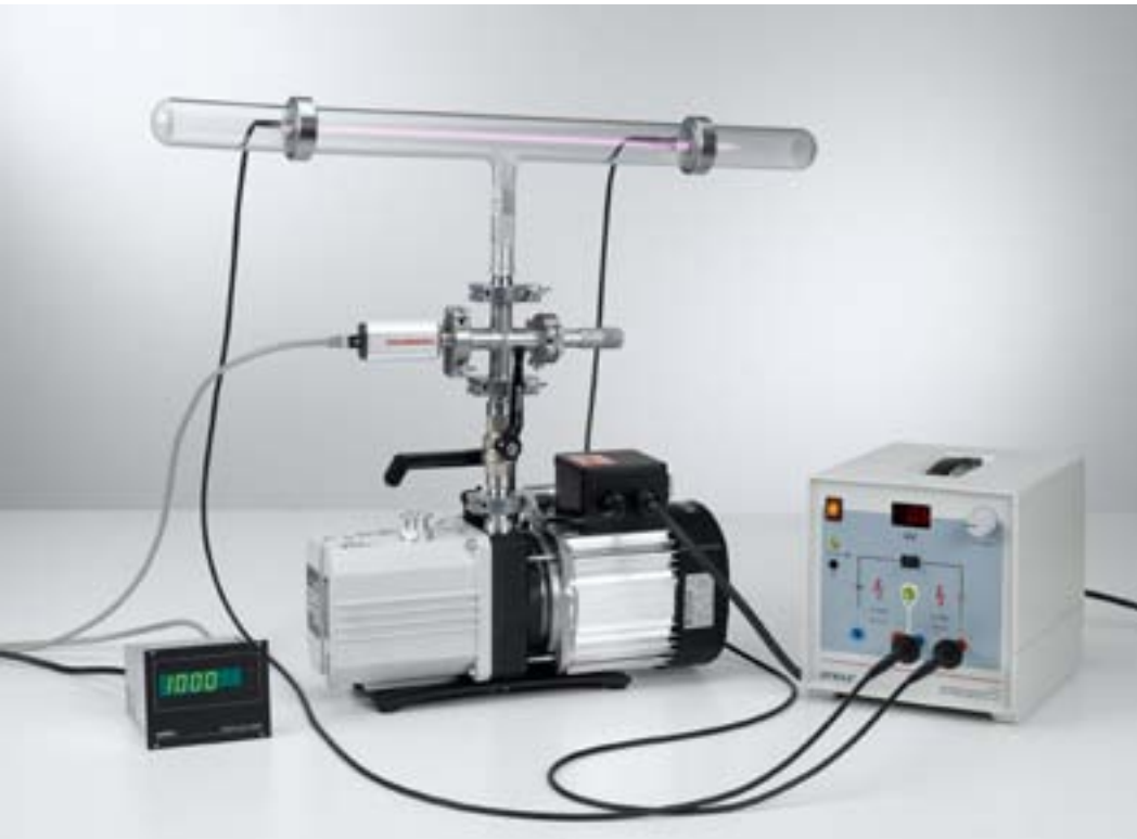
Magnetic deflection of cathode and canal rays (P3.9.3.1)
