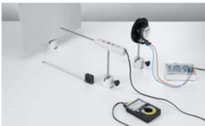
Determining the wavelength of standing sound waves (P1.7.3.2)
