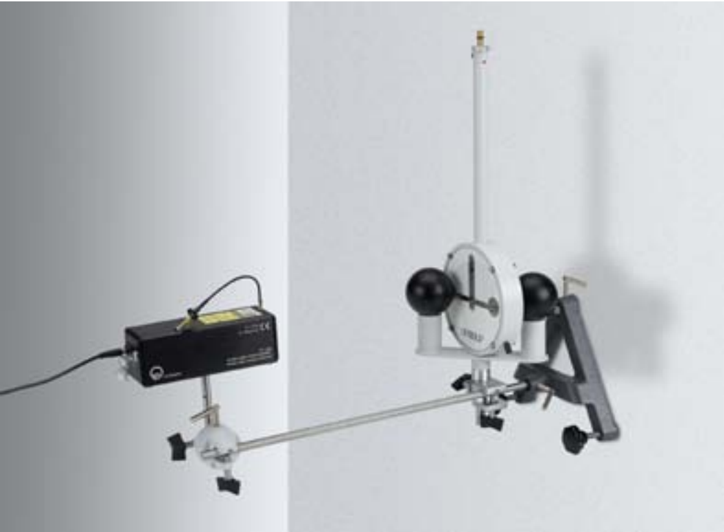
Determining the gravitational constant with the gravitation torsion balance after Cavendish - Measuring the excursion with a light pointer (P1.1.3.1)
