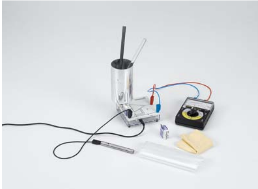
Basic electrostatics experiments with the electrometer amplifier (P3.1.1.2_a)
