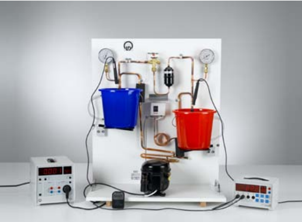
Determining the efficiency of the heat pump as a function of the temperature differential (P2.6.3.1_a)
