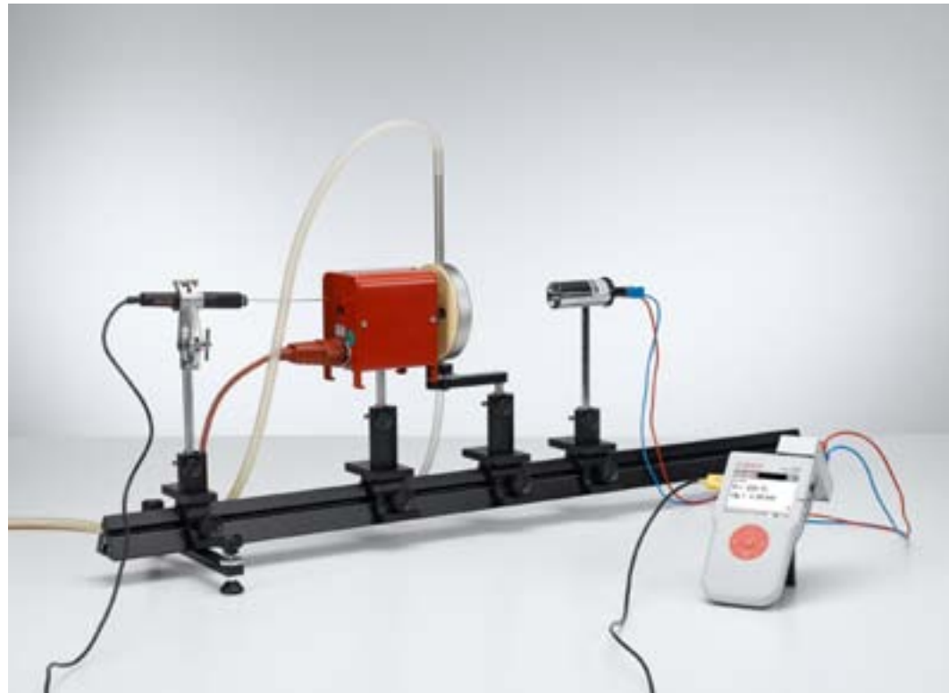
Stefan-Boltzmann law: measuring the radiant intensity of a „black body“ as a function of temperature (P5.5.2.1_b)
