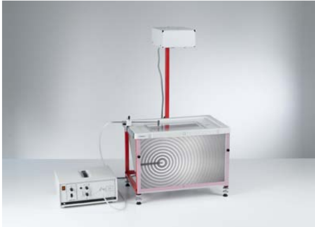
Exciting circular and straight water waves (P1.6.4.1)
