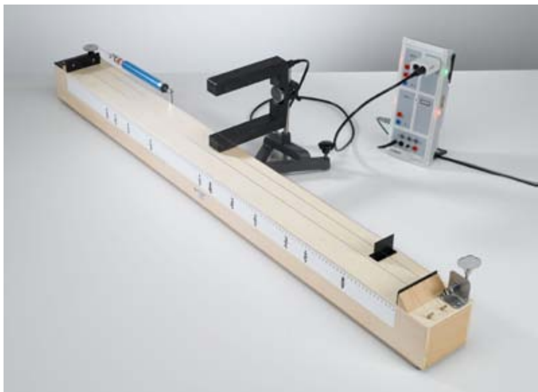
Determining the oscillation frequency of a string as a function of the string length and tension (P1.7.2.1)
