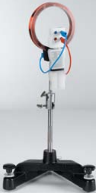
Measuring the earth's magnetic field with a rotating induction coil and wireless CASSY (P3.4.6.2)
