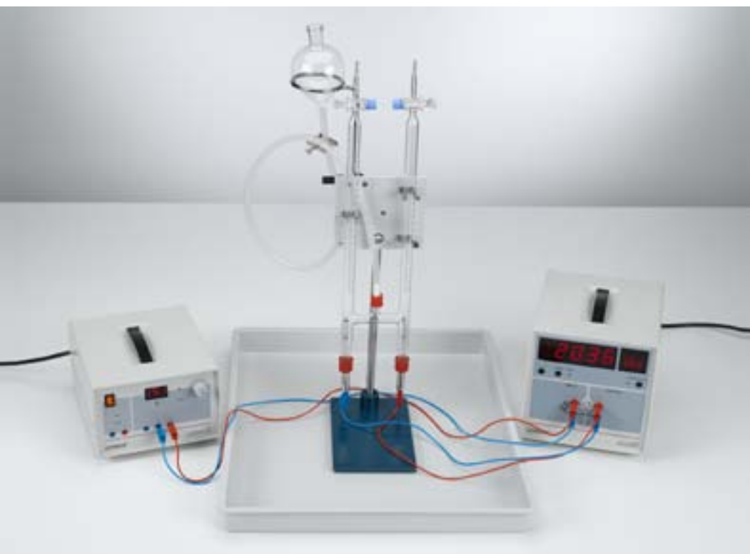
Determining the Faraday constant (P3.2.5.1)
