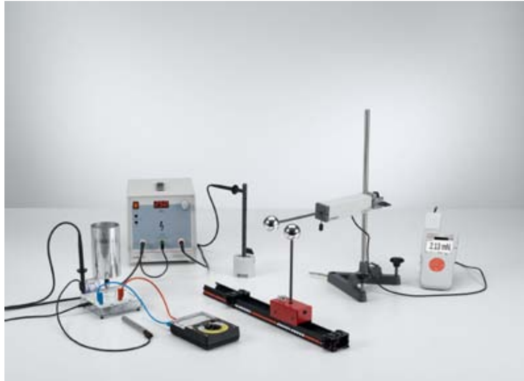
Confirming Coulomb's law - Measuring with the force sensor (P3.1.2.2_b)
