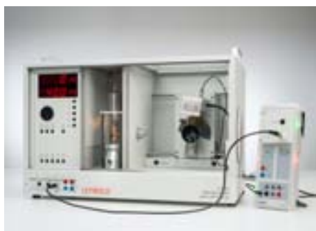
Recording and calibrating an X-ray energy spectrum
