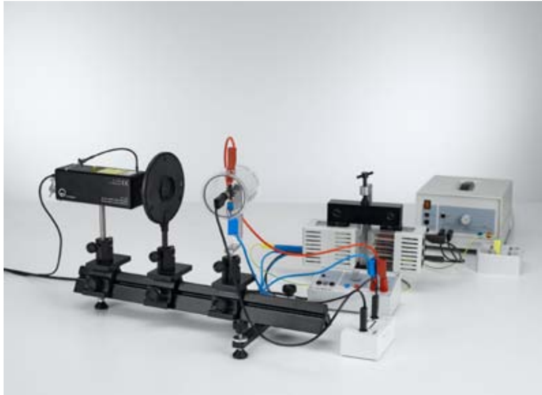
Observing individual lycopod spores in a Paul trap (P6.1.6.1_a)
