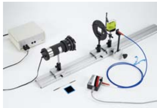
Absorption and fluorescence spectra of coloured liquids (P5.2.4.4)
