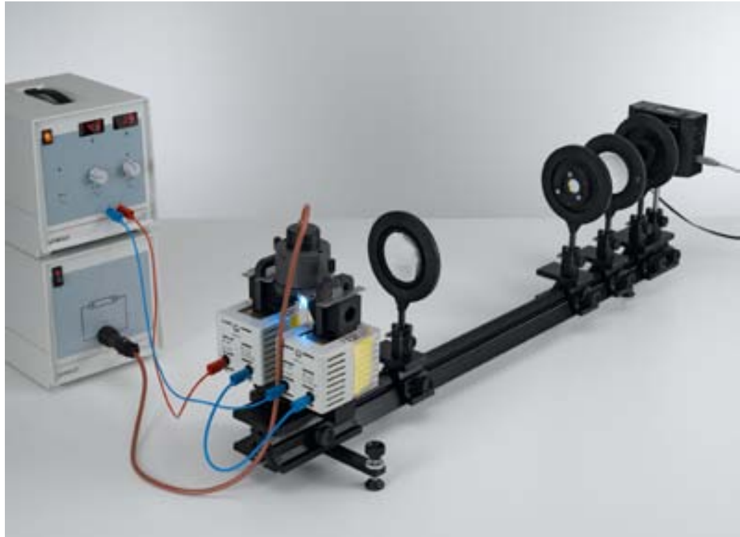
Measuring the Zeeman splitting of the red cadmium line as a function of the magnetic field - spectroscopy using a Fabry-Perot etalon (P6.2.7.4_b)
