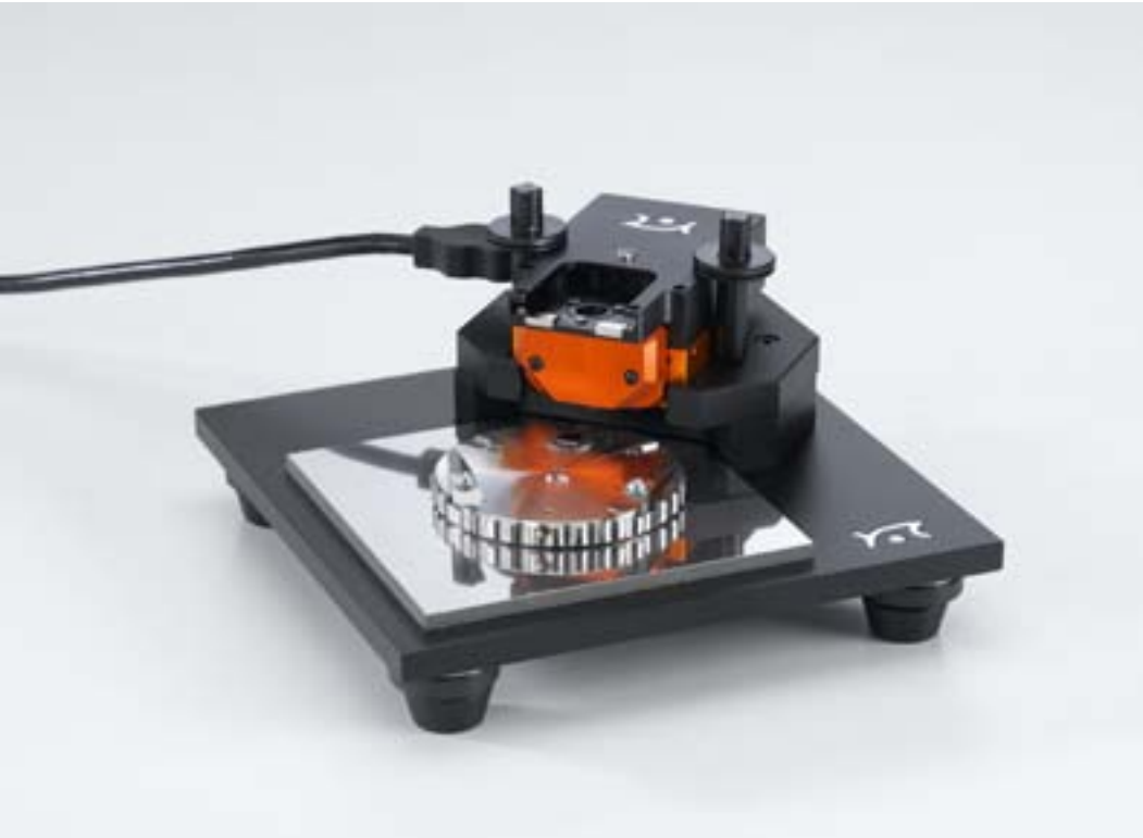
Investigating of surfaces using an atomic force microscope (AFM) (P7.4.1.4)
