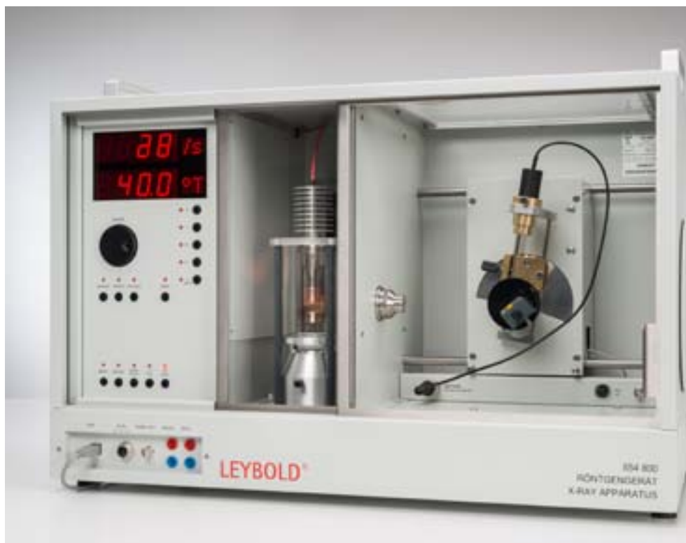
Fine structure of the characteristic X-ray radiation of a tungsten anode (P6.3.6.5)
