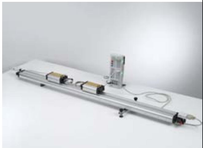
Newton's third law and laws of collision - Recording and evaluating with two ultrasonic motion sensors and CASSY (P1.3.4.5)
