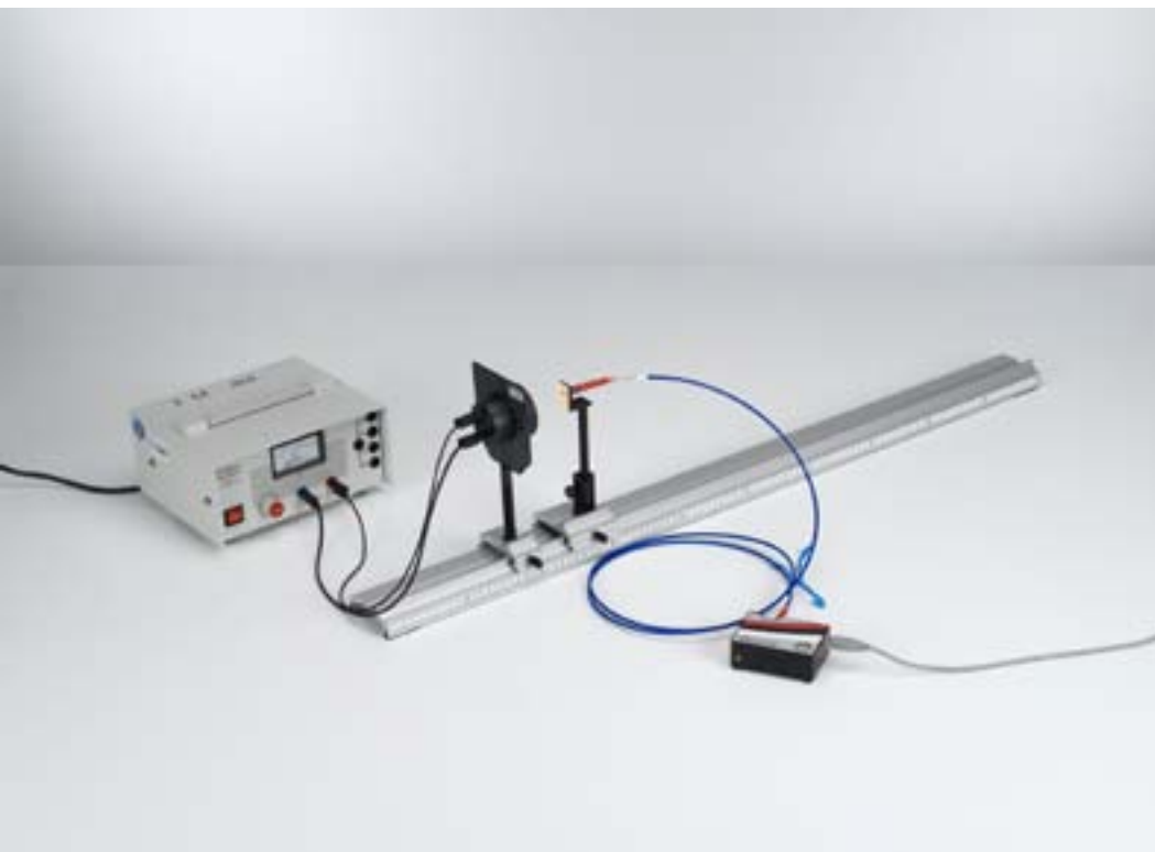
The Wien's displacement law - spectral recording of the black body radiation (P5.5.2.4)
