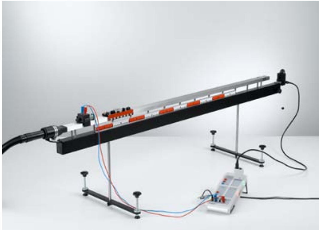
Path-time and velocity-time diagrams of straight motion - Recording and evaluating with CASSY (P1.3.3.4)
