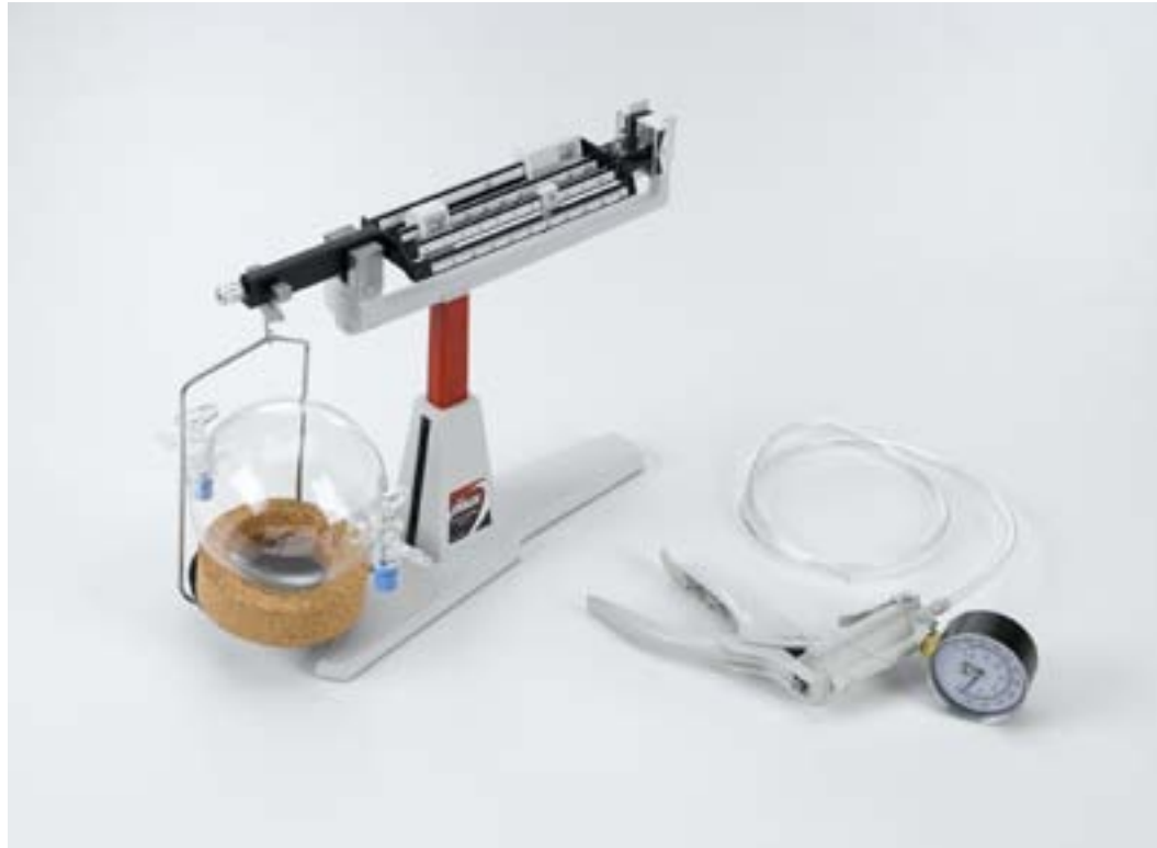
Determining the density of air (P1.1.2.4)
