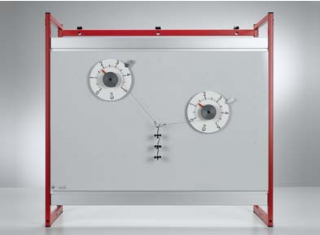
Composition and resolution of forces (P1.2.2.1_b)
