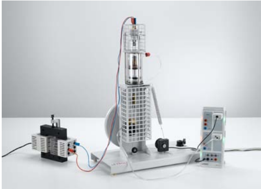
pV diagram of the hot-air engine as a heat engine - Recording and evaluating with CASSY (P2.6.2.4)
