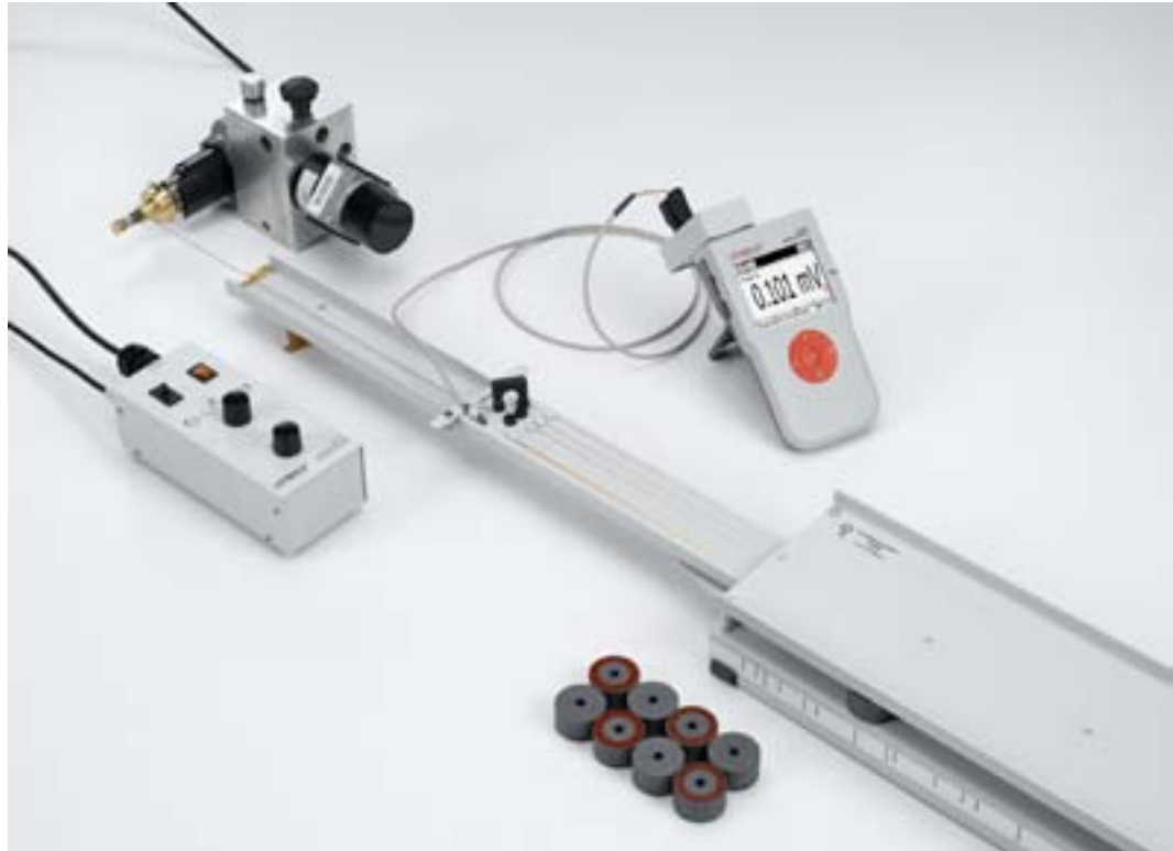
Measuring the induction voltage in a conductor loop moved through a magnetic field (P3.4.2.1_b)
