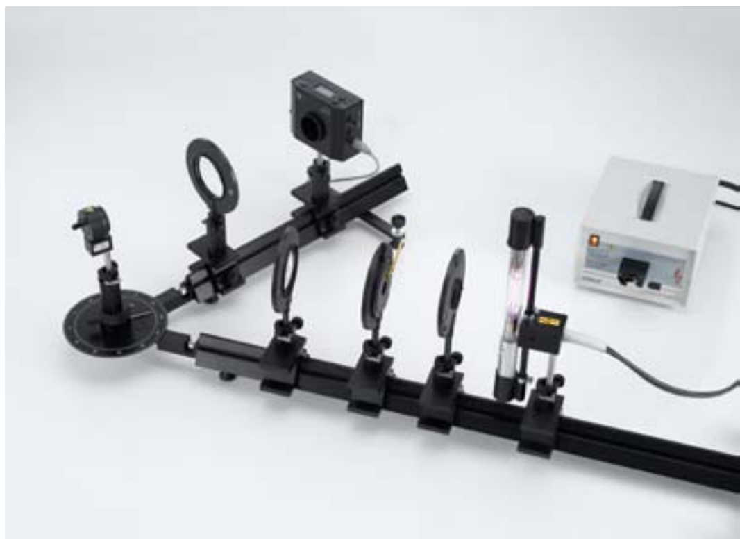
Observing the splitting of the Balmer series on deuterated hydrogen (isotope splitting) (P6.2.1.3_b)
