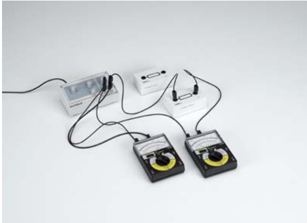
Frequency response and form factor of a multimeter (P3.6.5.1)
