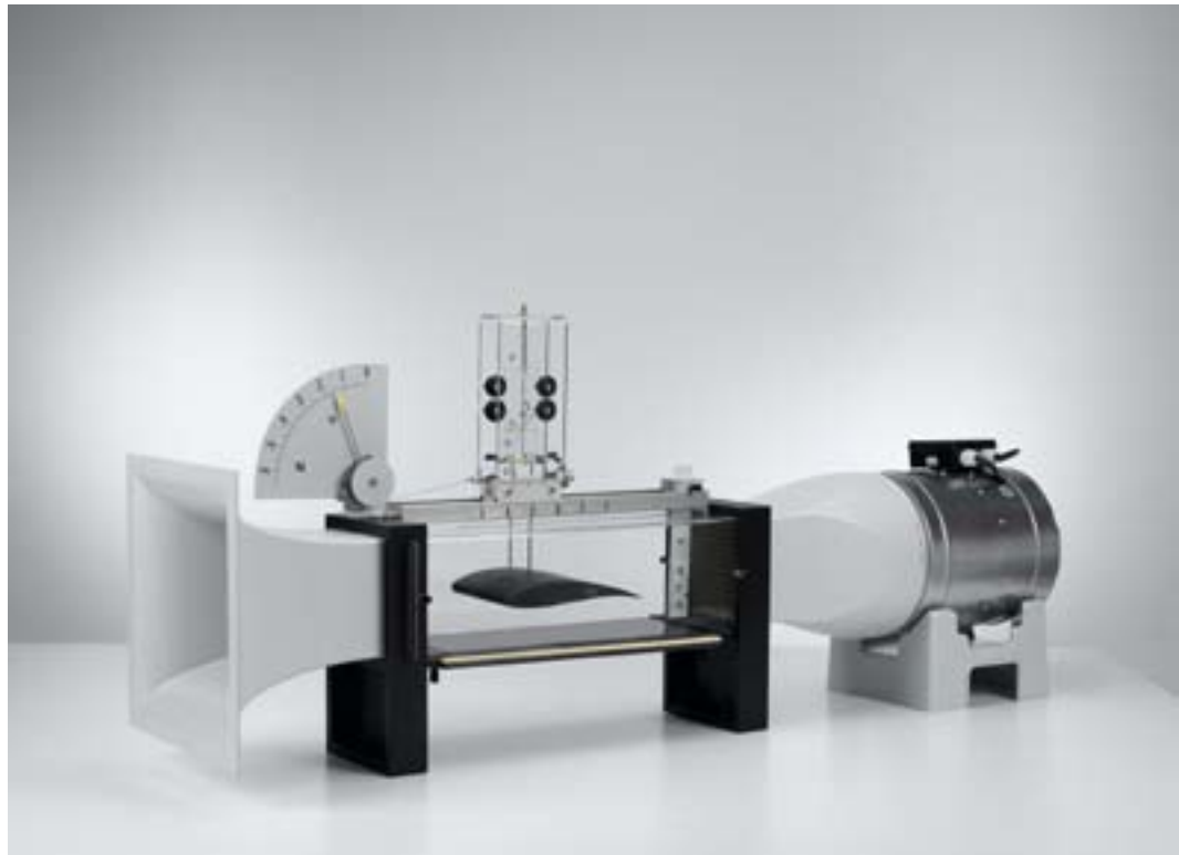
Recording the airfoil profile polars in a wind tunnel (P1.8.7.1)
