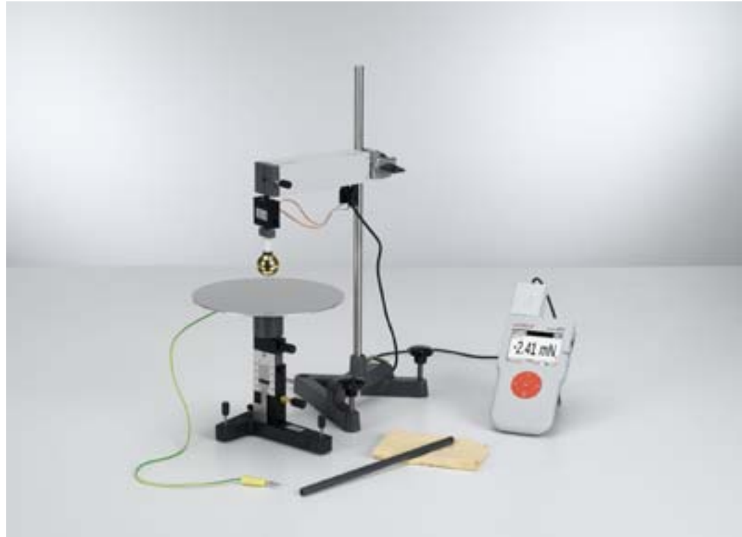
Measuring the force between a charged sphere and a metal plate (P3.1.4.3_b)
