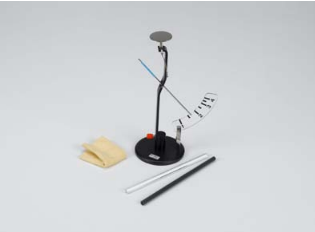
Basic electrostatics experiments with the field electrometer (P3.1.1.1)
