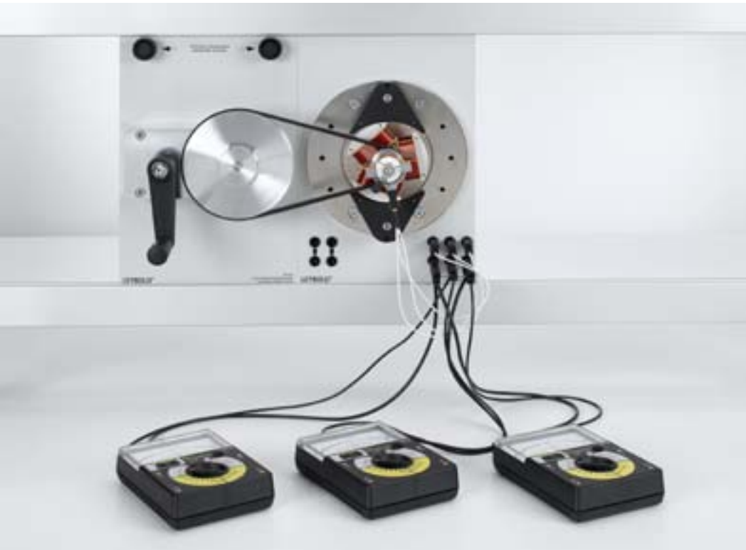
Experiments with a three-phase revolving-armature generator (P3.5.4.1_b)
