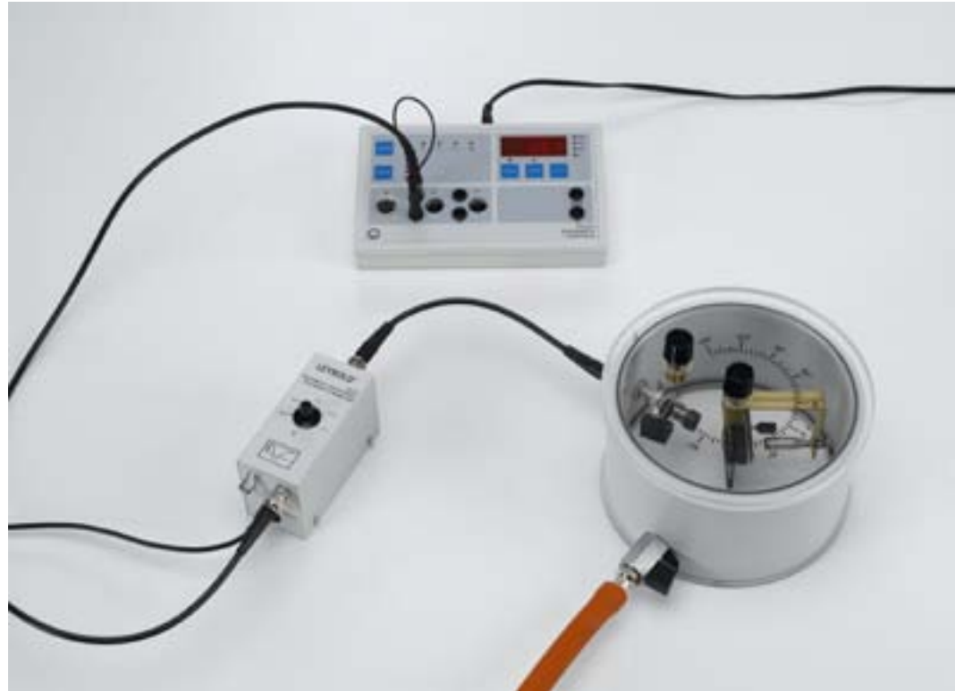
Rutherford scattering: measuring the scattering rate as a function of the scattering angle and the atomic number (P6.5.2.1)
