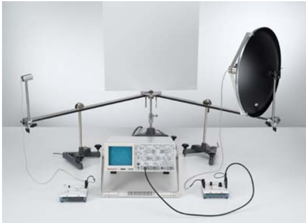
Reflection of planar ultrasonic waves at a plane surface (P1.7.4.1)
