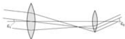
Ray path through the Kepler telescope
