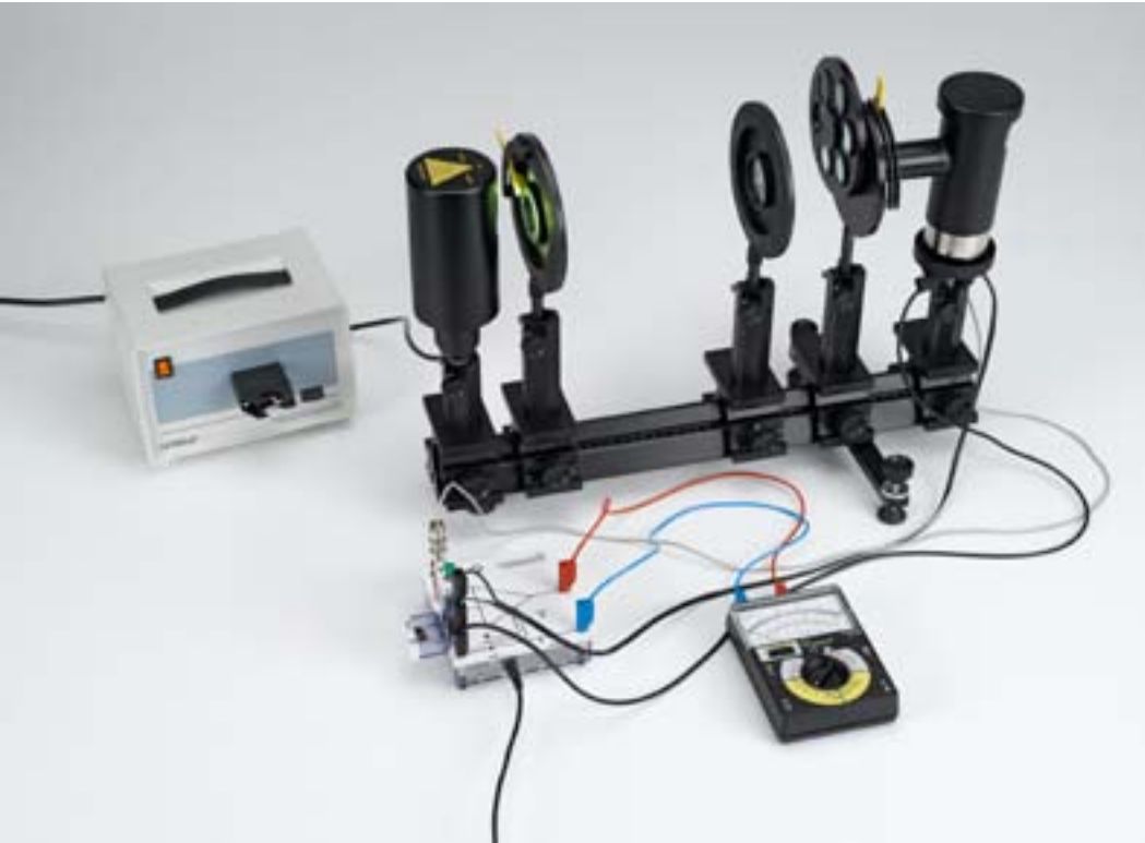
Determining Planck's constant - Selection of wavelengths using interference filters on the optical bench (P6.1.4.3_a)
