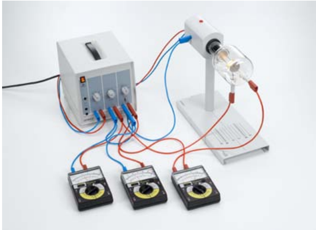
Discontinuous energy emission of electrons in a gas-filled triode (P6.2.3.1)
