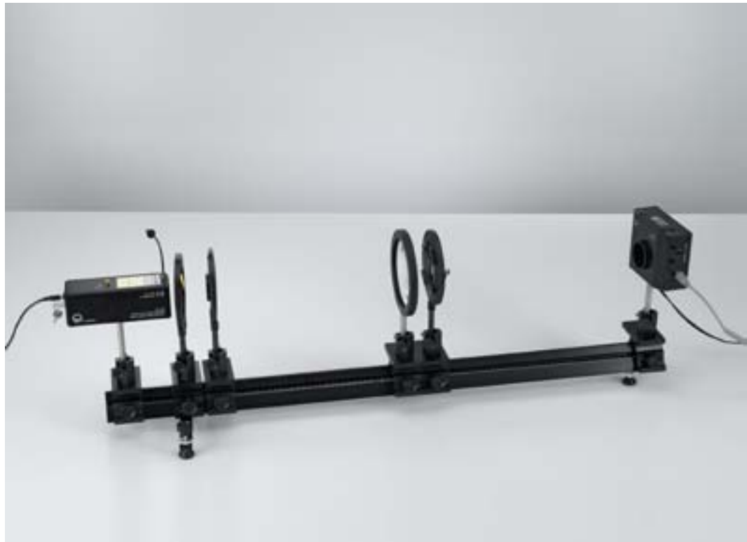
Diffraction at a half-plane - Recording and evaluating with VideoCom (P5.3.1.8)
