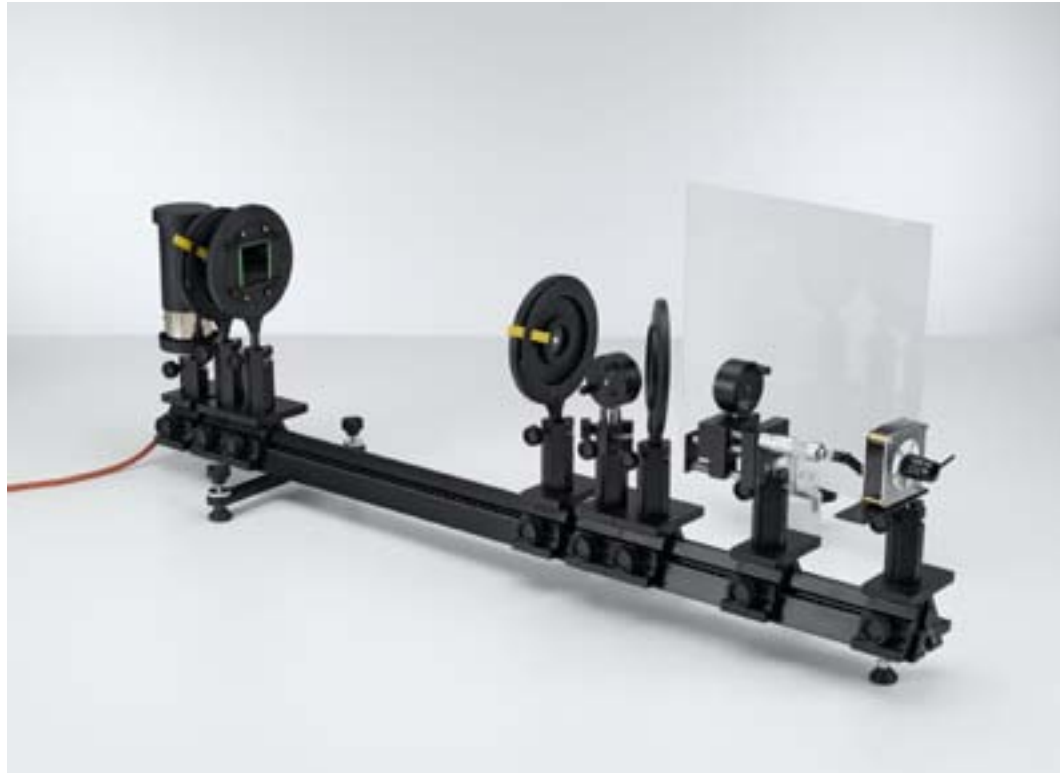
Determination of the coherence time and the line width of spectral lines with the Michelson interferometer (P5.3.4.4_a)
