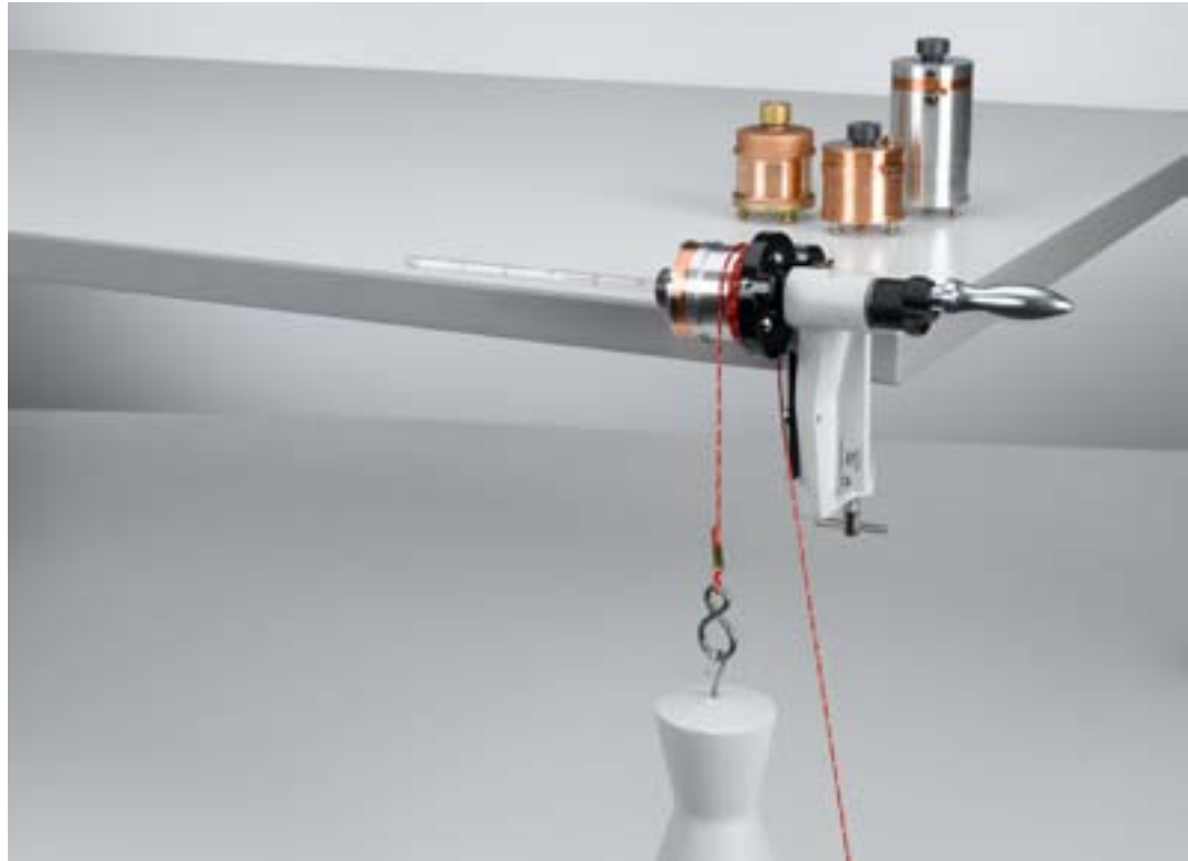
Converting mechanical energy into heat energy - Recording and evaluating measured values manually (P2.3.3.1_a)
