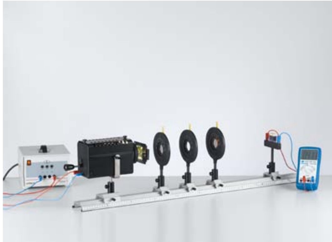
Quarter-wavelength and half-wavelength plate (P5.4.2.2_b)
