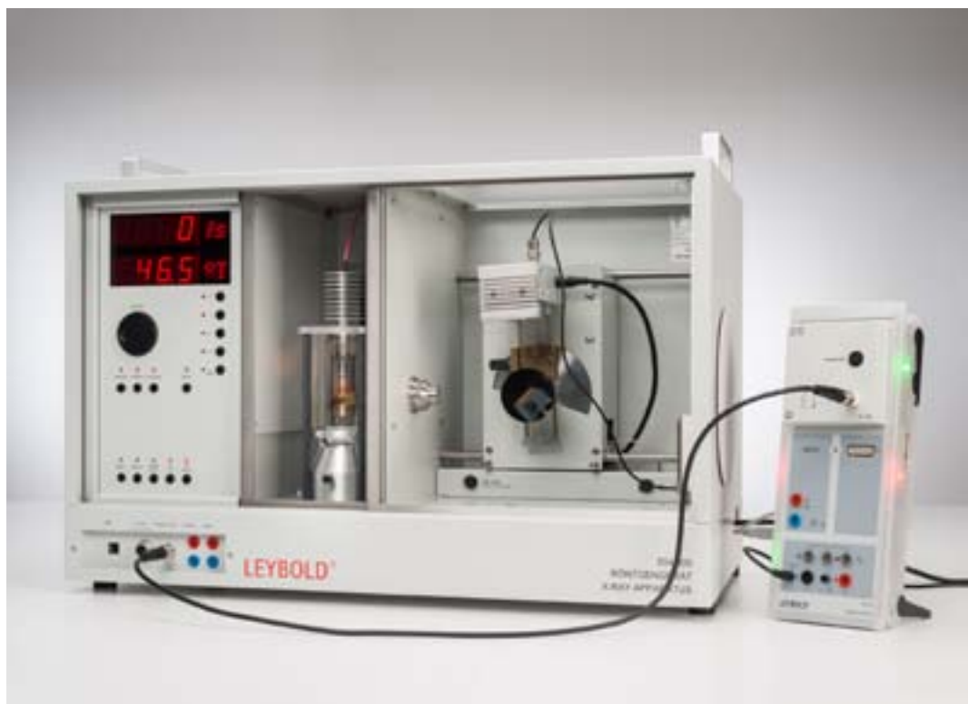
Application of X-ray fluorescence for the non-destructive analysis of the chemical composition (P7.5.1.1)
