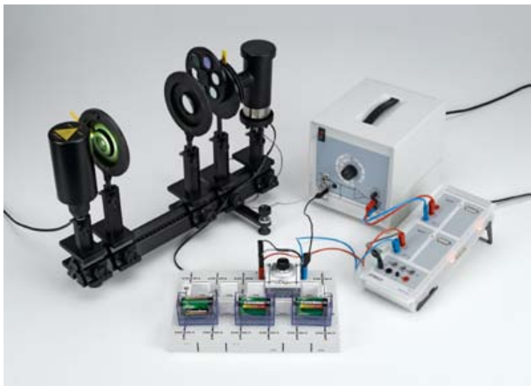
Determining Planck's constant - Recording the current-voltage characteristics, selection of wavelengths using interference filters on the optical bench (P6.1.4.4_b)
