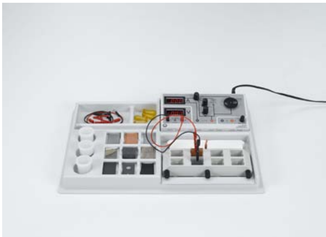
Measuring the voltage at simple galvanic elements (P3.2.6.2)
