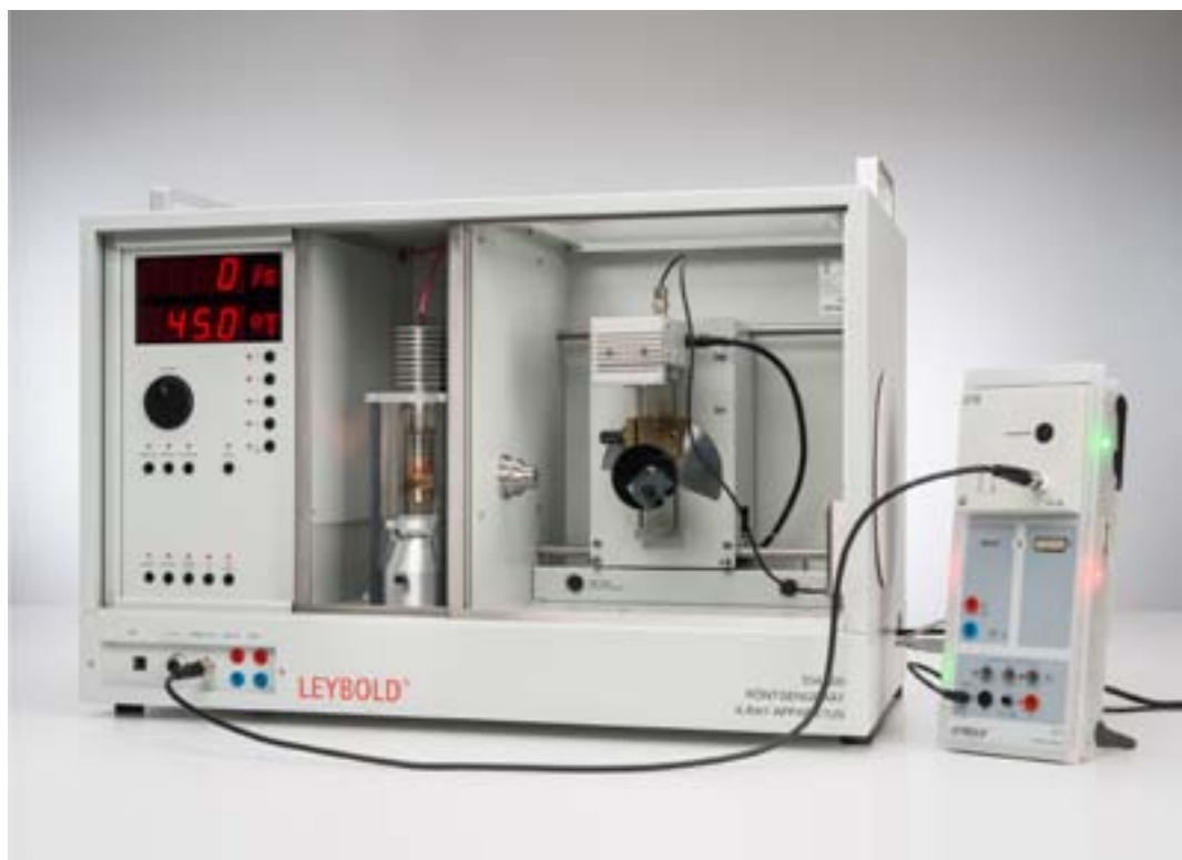
Compton effect: Measurement the energy of the scattered photons as a function of the scattering angle (P6.3.7.2)
