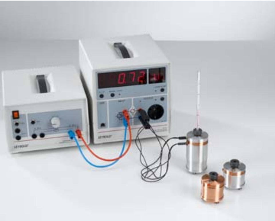
Converting electrical energy into heat energy - Measuring with the joule and wattmeter (P2.3.4.2_a)
