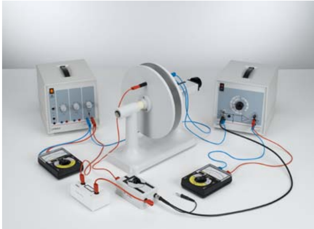
Determining the capacitance of a plate capacitor – Measuring the charge with the I-measuring amplifier D (P3.1.7.3)
