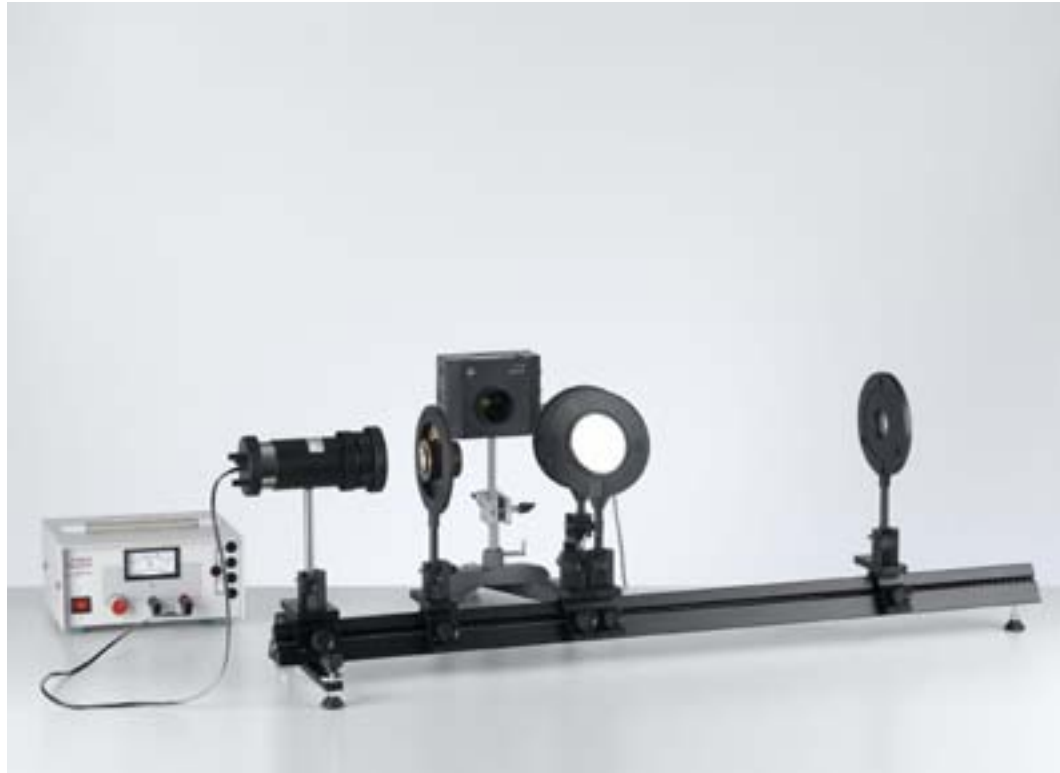
Newton's rings in reflected monochromatic light - Recording and evaluating with VideoCom (P5.3.3.3)
