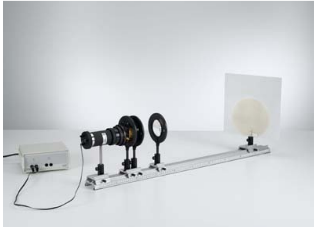
Magnifier and microscope (P5.1.4.1_b)
