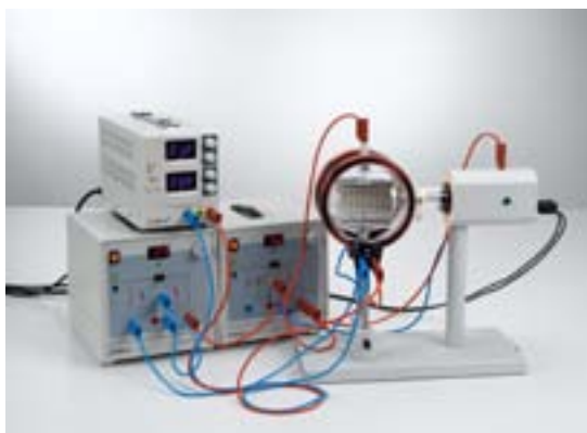
Investigating the deflection of electrons in magnetic fields
