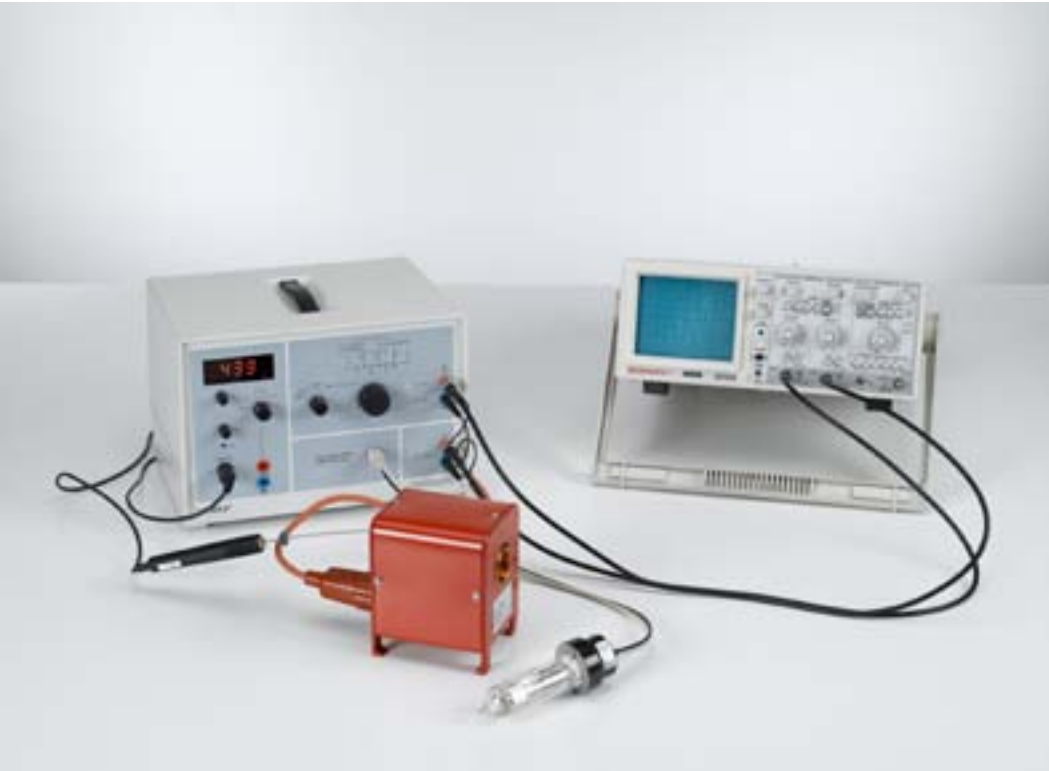
Franck-Hertz experiment with mercury - Recording with the oscilloscope (P6.2.4.1_b)
