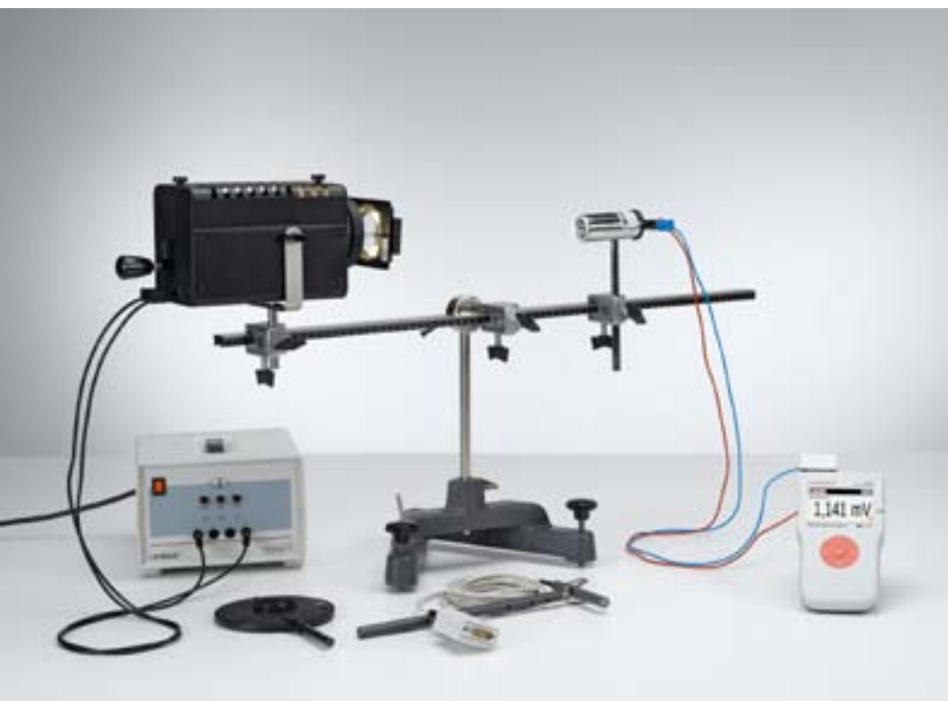
Determining the radiant flux density and the luminous intensity of a halogen lamp (P5.5.1.1_a)
