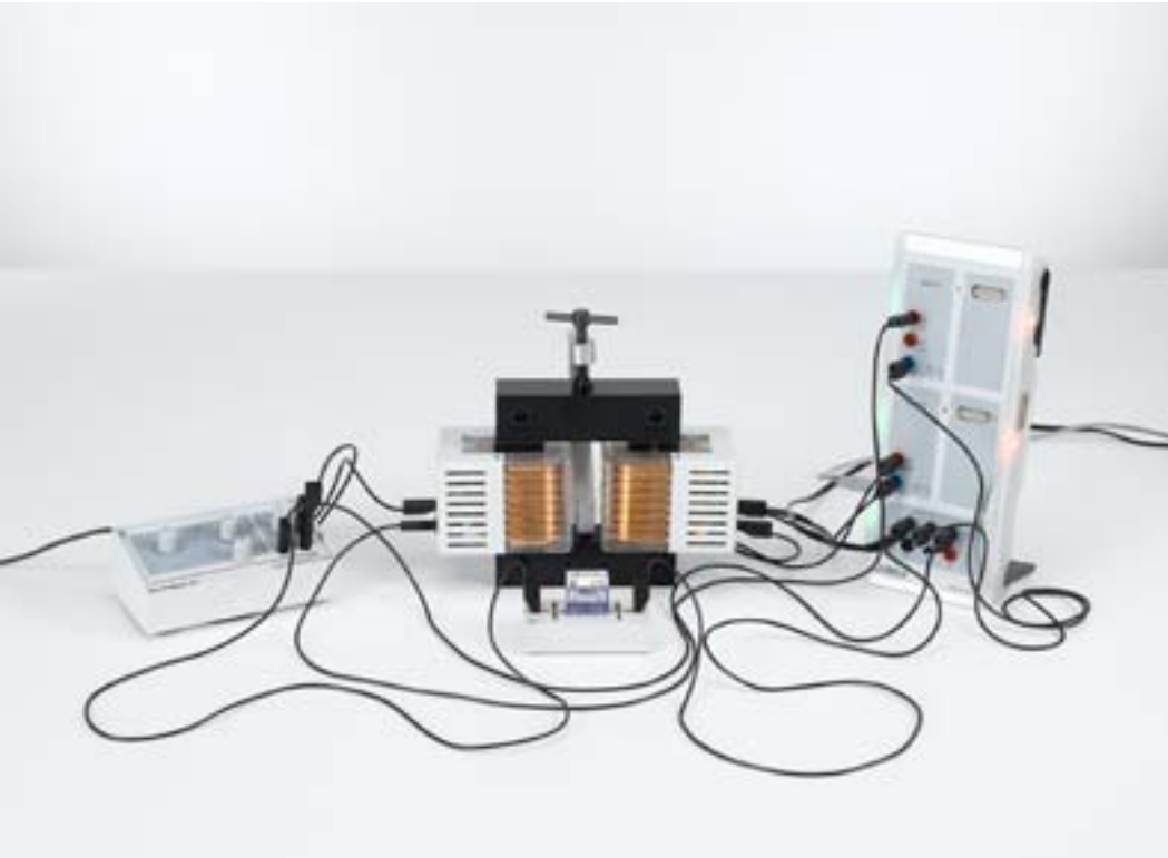
Recording the initial magnetization curve and the hysteresis curve of a ferromagnet (P7.3.2.1_a)
