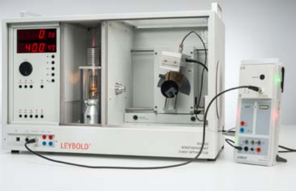
Recording and calibrating an X-ray energy spectrum (P6.3.5.1)
