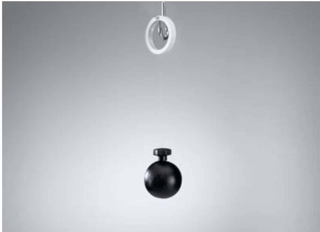
Determining the gravitational acceleration with a simple pendulum (P1.5.1.1_a)
