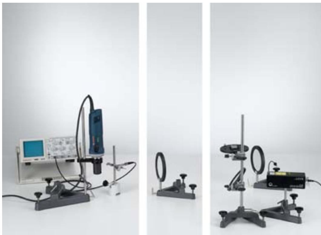
Determining the velocity of light by means of the rotating-mirror method according to Foucault and Michelson - Measuring the image shift as a function of the rotational speed of the mirror (P5.6.1.1)
