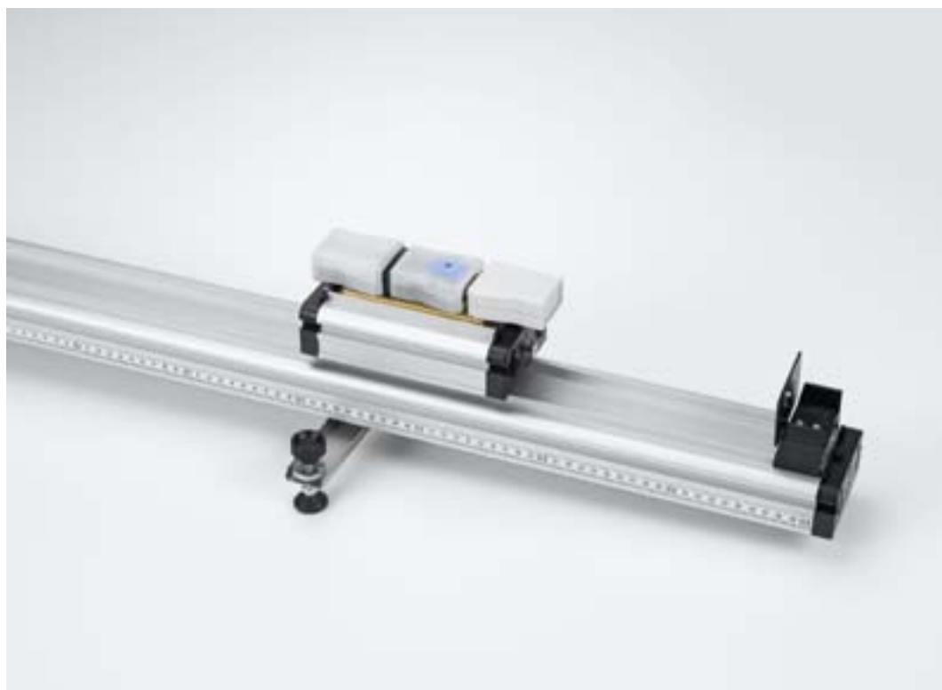
Accelerated motions with an acceleration sensor (P1.3.2.5)
