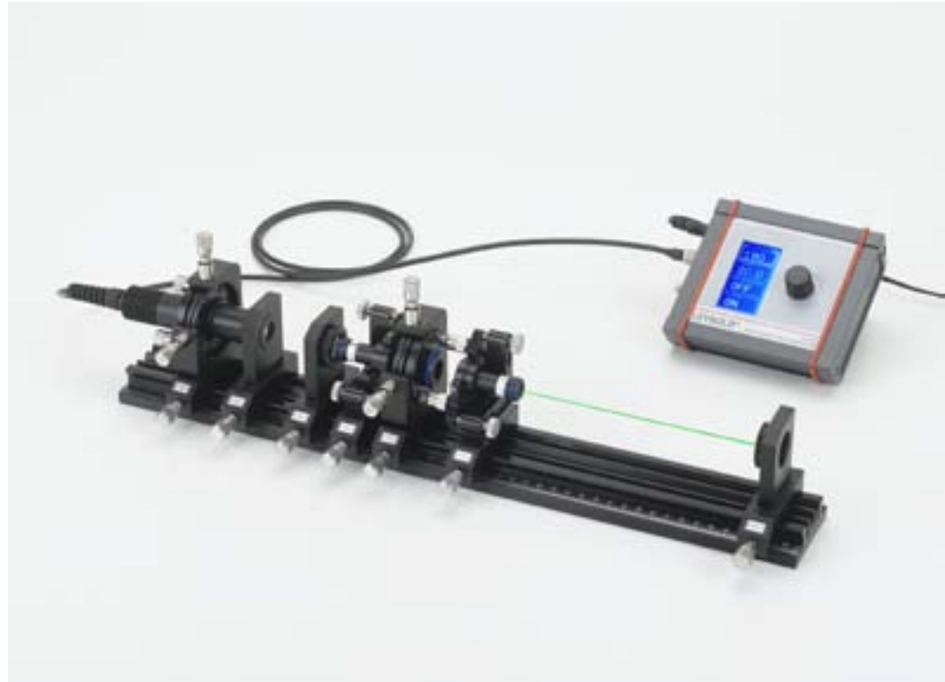
Frequency doubling, 1064 nm → 532 nm (P5.8.6.3)
