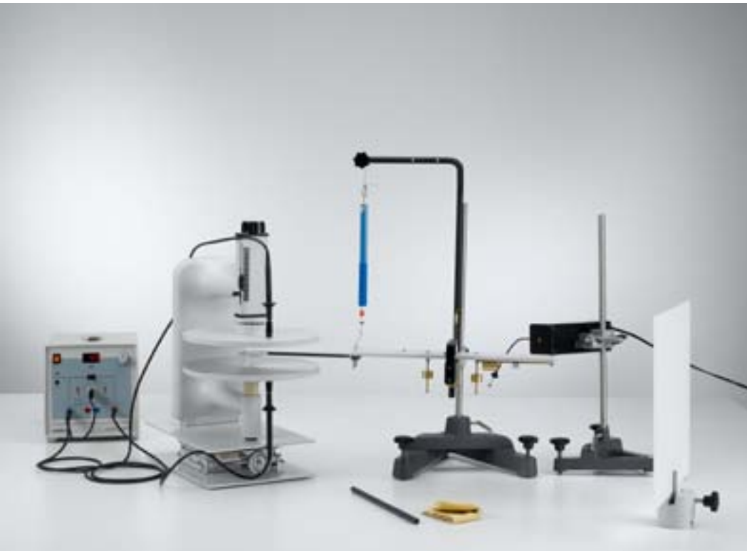
Measuring the force of an electric charge in a homogeneous electric field (P3.1.4.1)
