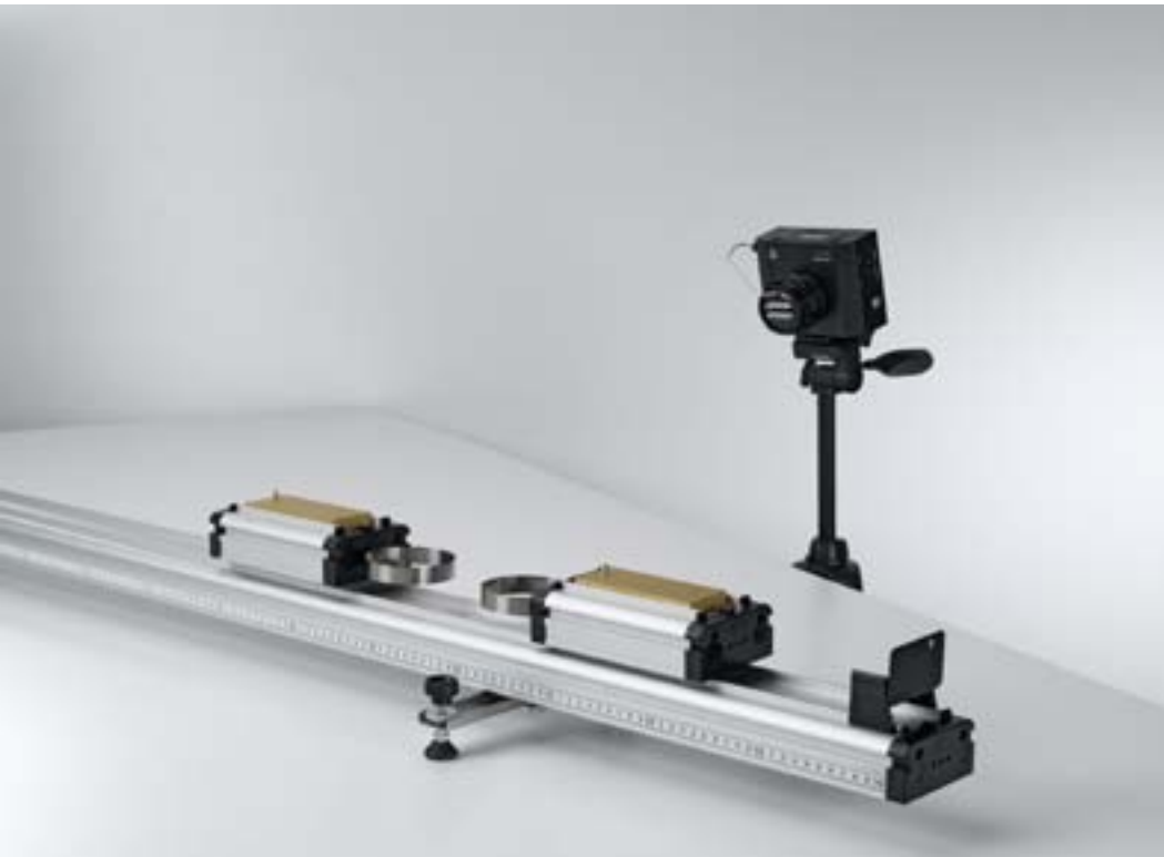
Newton's third law and laws of collision - Recording and evaluating with VideoCom (P1.3.4.4_a)
