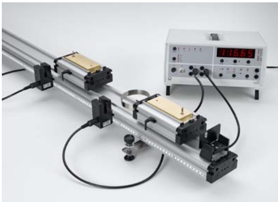
Energy and linear momentum in elastic collision - Measuring with two forked light barriers (P1.3.4.1_c)
