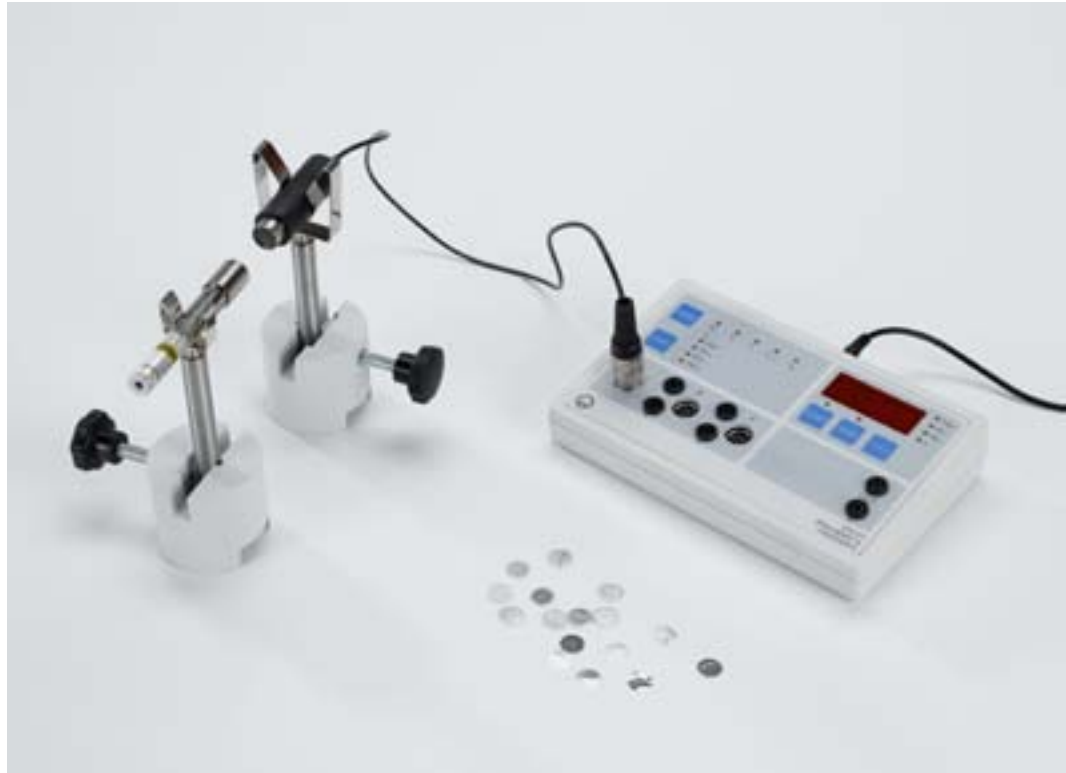
Attenuation of \beta radiation when passing through matter (P6.4.4.2)
