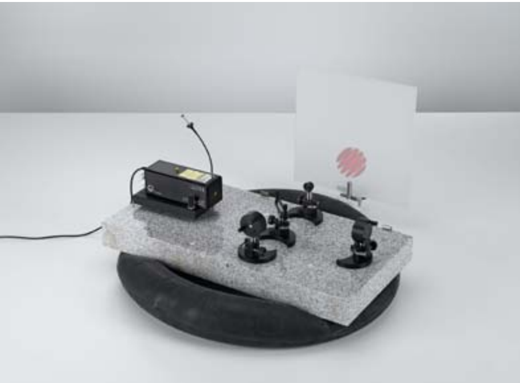
Setting up a Michelson interferometer on the laser optics base plate (P5.3.4.1)
