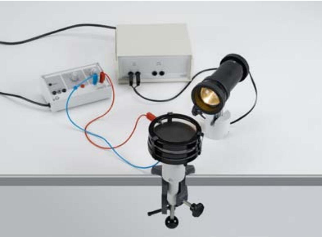
Demonstrating the tracks of \alpha particles in a Wilson cloud chamber (P6.5.1.1)
