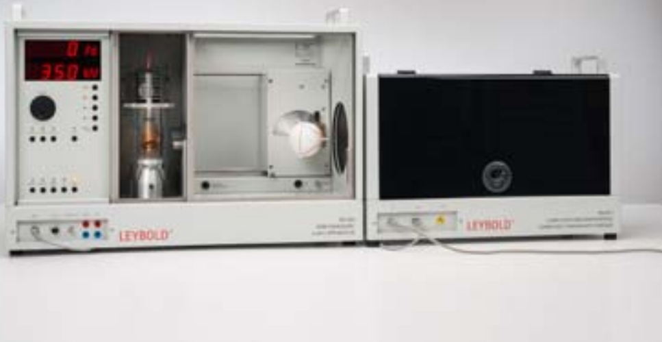
Measurement and presentation of a computed tomogram with the computed tomography module (P6.3.8.1)
