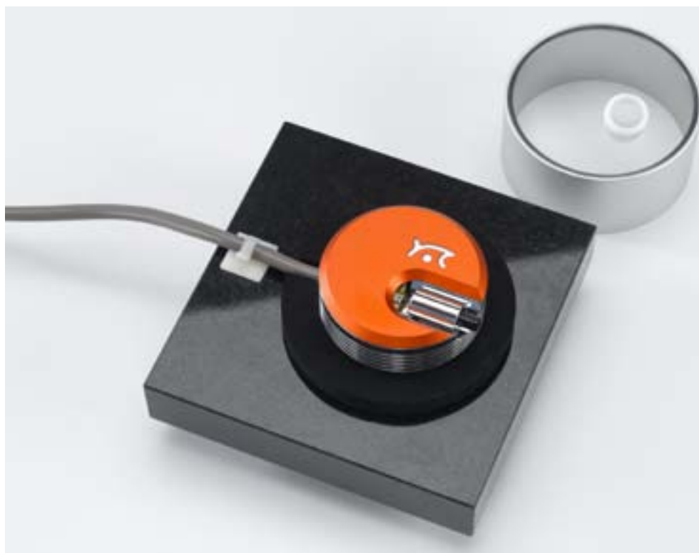
Investigating a graphite surface using a scanning tunneling microscope (P7.4.1.1)
