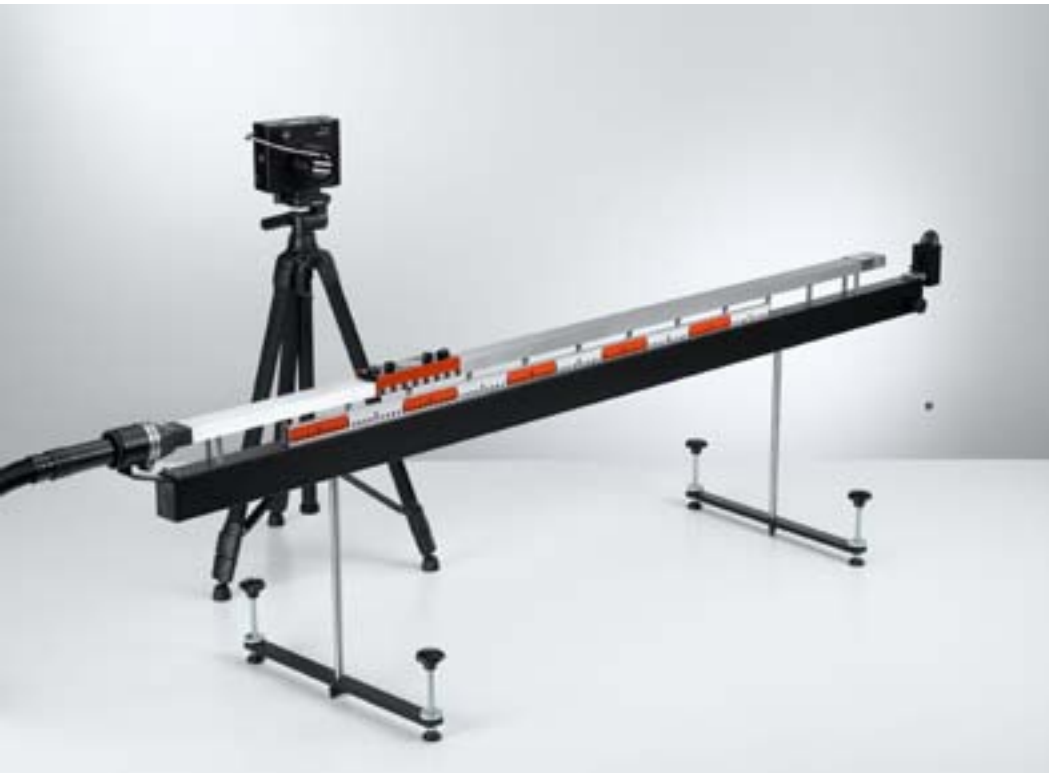
Confirming Newton's first and second laws for linear motions - Recording and evaluating with VideoCom (P1.3.3.7)
