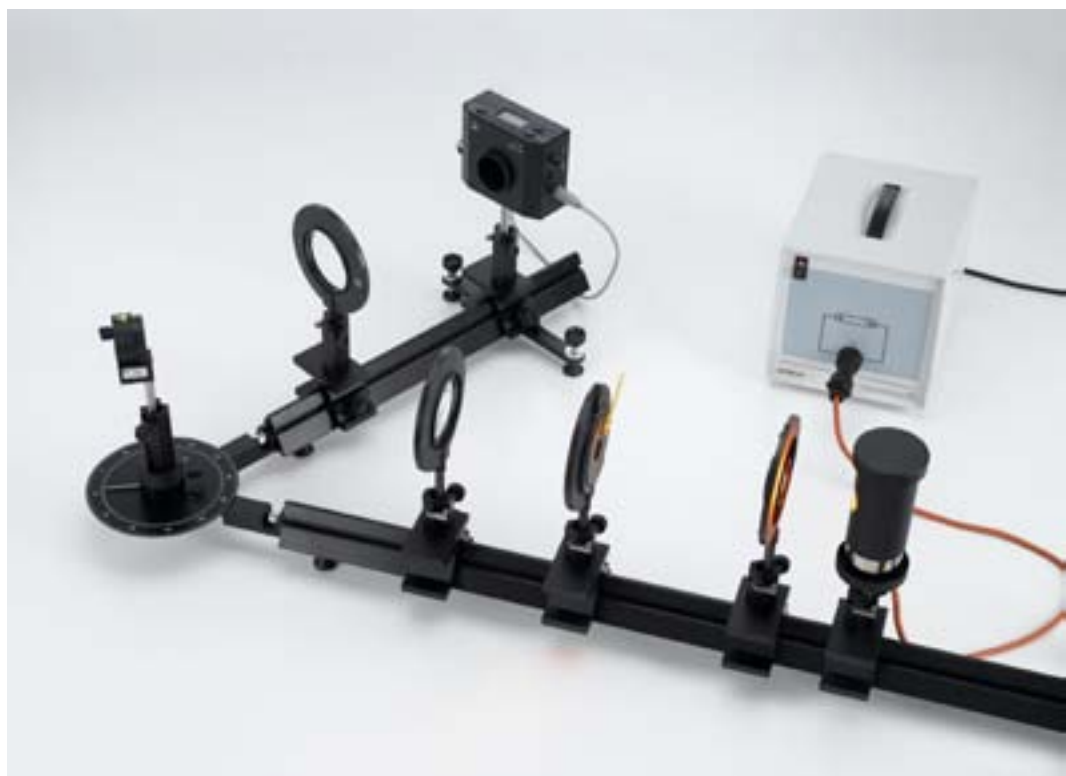
Investigating the spectrum of a high pressure mercury lamp (P6.2.2.3_c)
