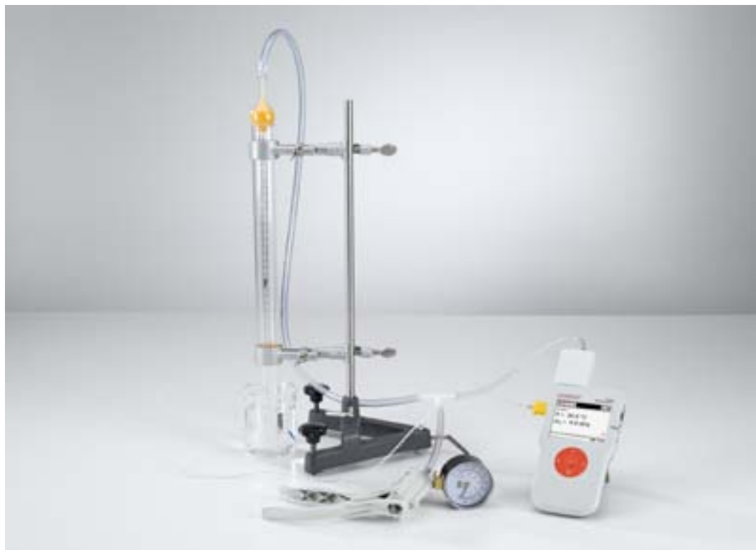
Temperature-dependency of the volume of a gas at a constant pressure (Gay-Lussac's law) (P2.5.2.2_c)
