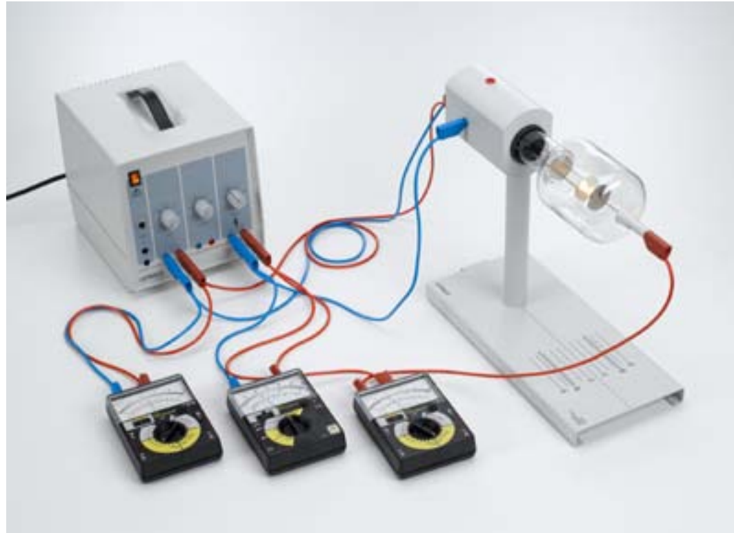
Recording the characteristic of a tube diode (P3.8.1.1)
